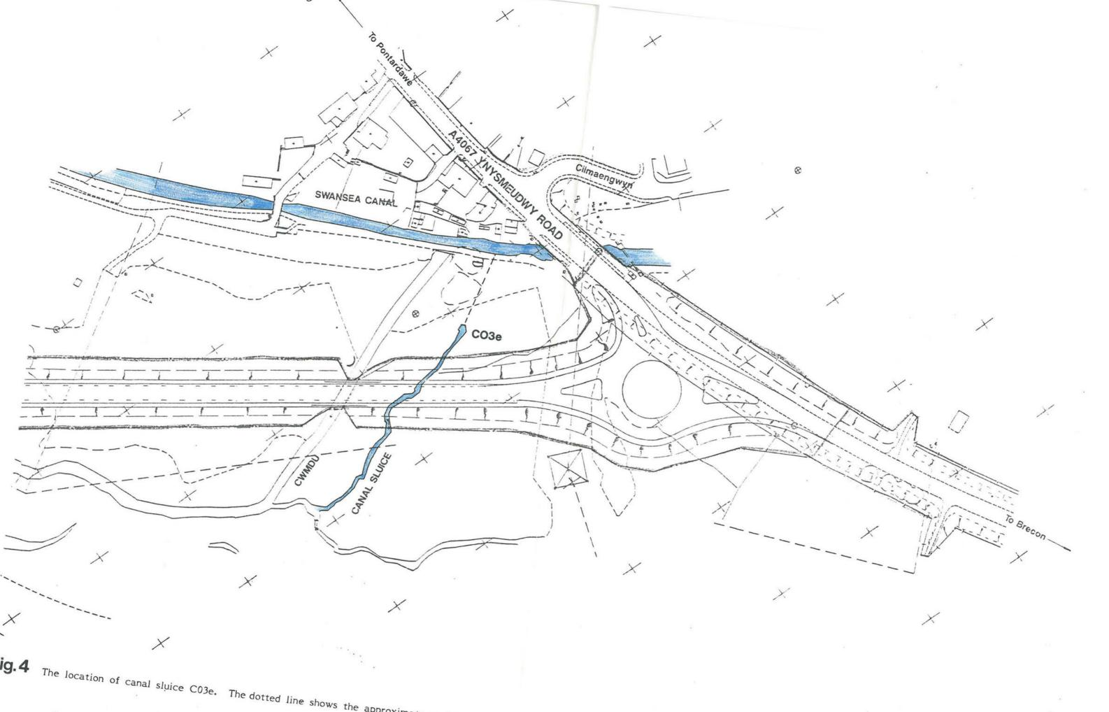
ig.4 The location of canal sluice C03e. The dotted line shows the approximate position of the culverted section.
