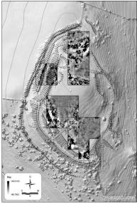
Figure 6 (left): resistivity data (Twin 0.5), (right): resistivity data (Double-Dipole) both overlain on hachure survey.
