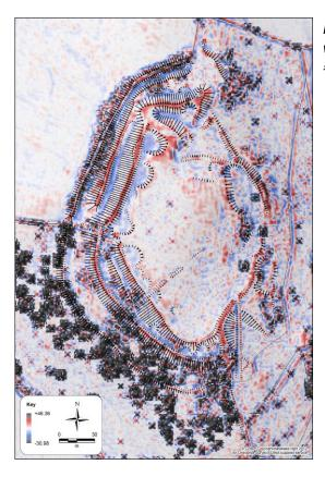
Figure 4. Mean curvature derived from LiDAR data with topographic survey overlain (red = convex, blue = concave).
