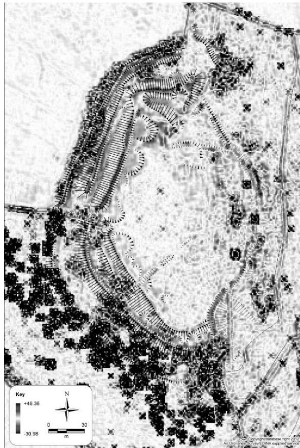
Figure 4. Mean curvature derived from LiDAR data overlain on topographic data.
