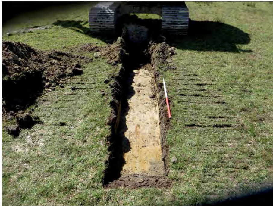
Plate 5: Representative trial pit from Section 1 (TPA2)
