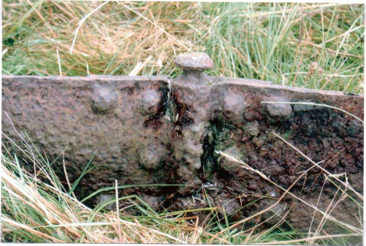
Photo 23. One of three joints in the brake band of the Cae Abatty Tramway winding drum.
