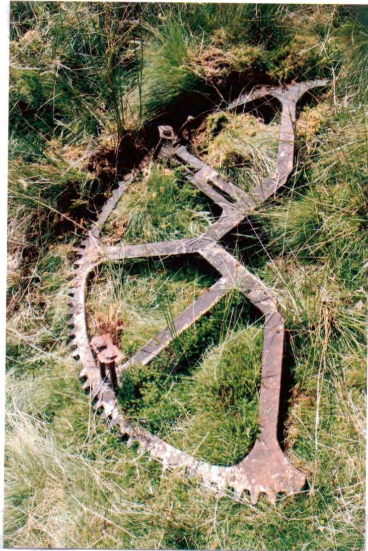
Photo 32. One of two pairs of bolts on the periphery of the large gearwheel. Four pairs of bolts would have fixed it to one spider of the winding drum.
