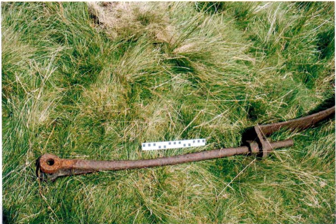
Photo 20. Pull rod on the end of the brake band for the winding drum of the Cae Abatty Tramway.
