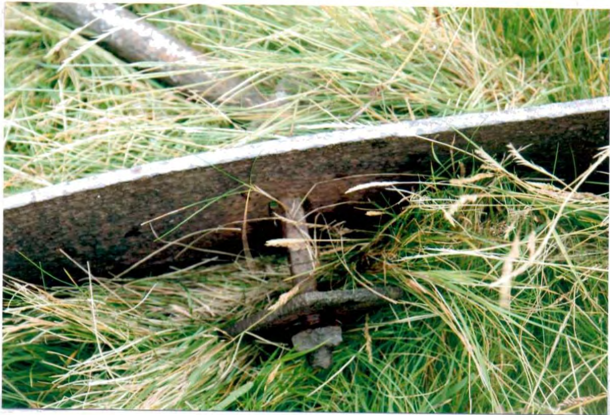
Photo 22. Detail of the braking surface rim, showing one of the bolts which attached it to the surface of the drum.
