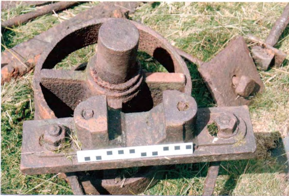
Photo 27. The second bearing blocks found at the summit of the Cae Abatty Tramway, with the axle end cap beyond. Comparison with the bearing blocks on the Cae Abatty Quarry drumhouse suggests that this one was a winch bearing, which was provided with brass bearings.
