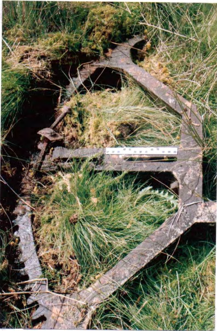
Photo 34. Detail of the centre hole in the large gearwheel. The centre of the gearwheel would have fitted a 0.33m (15") square axle.
