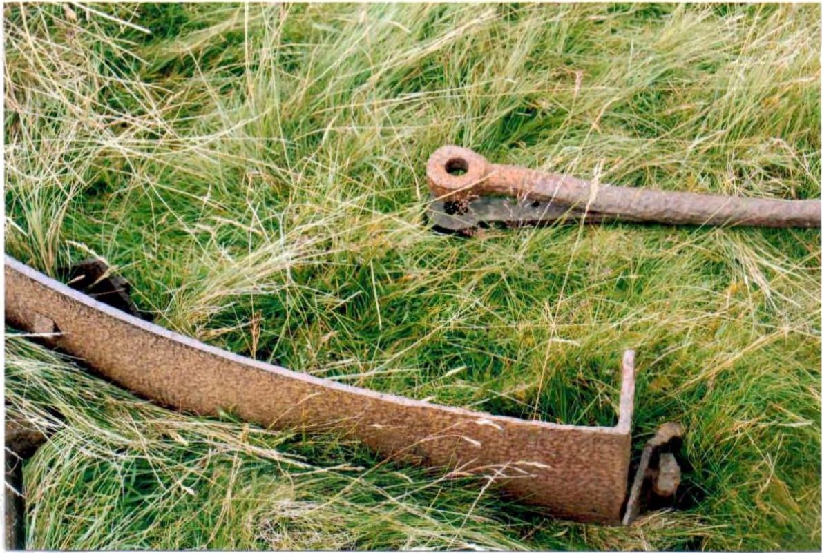
Photo 21. End of the section of braking surface rim of the Cae Abatty Tramway winding drum, showing the bolted flange joining the next section. Brake band pull rod beyond.
