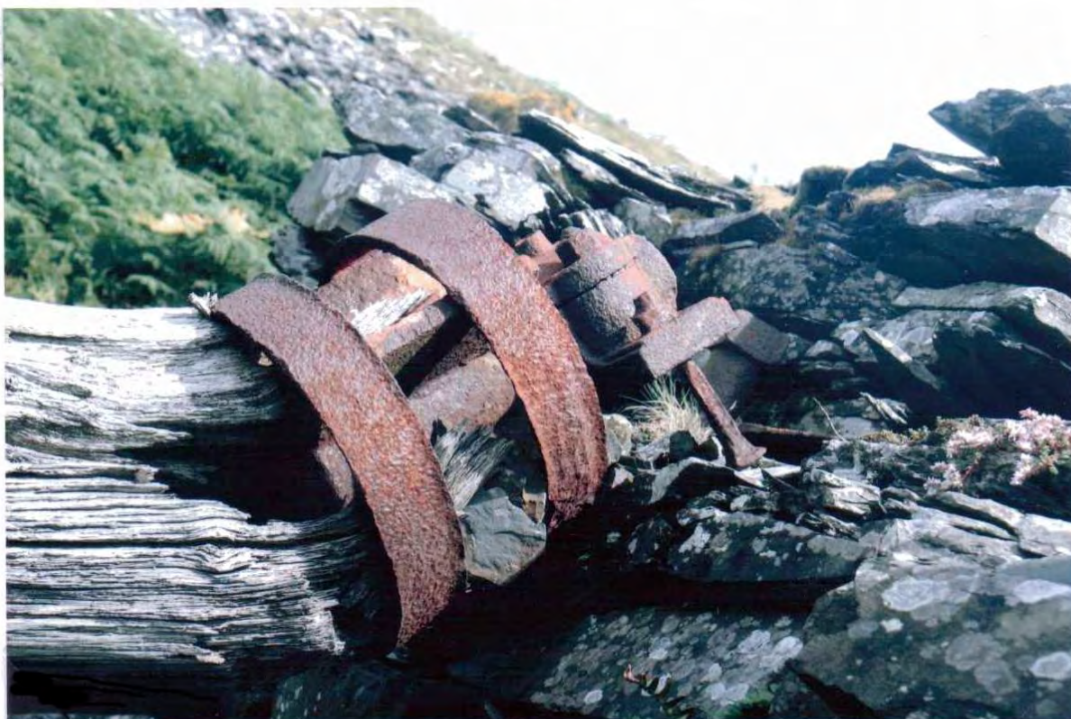
Photo 6. The East axle end cap of the Cae Abatty Quarry Incline Drum, with the journal still in the displaced bearing block.
