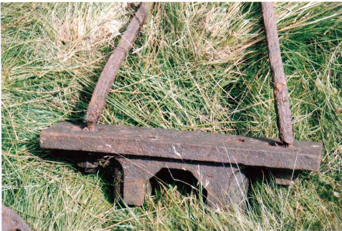
Photo 28. The winch bearing block, with holding down bolts still in place. These indicate that the timbers which carried it were about 0.4m (16") deep.
