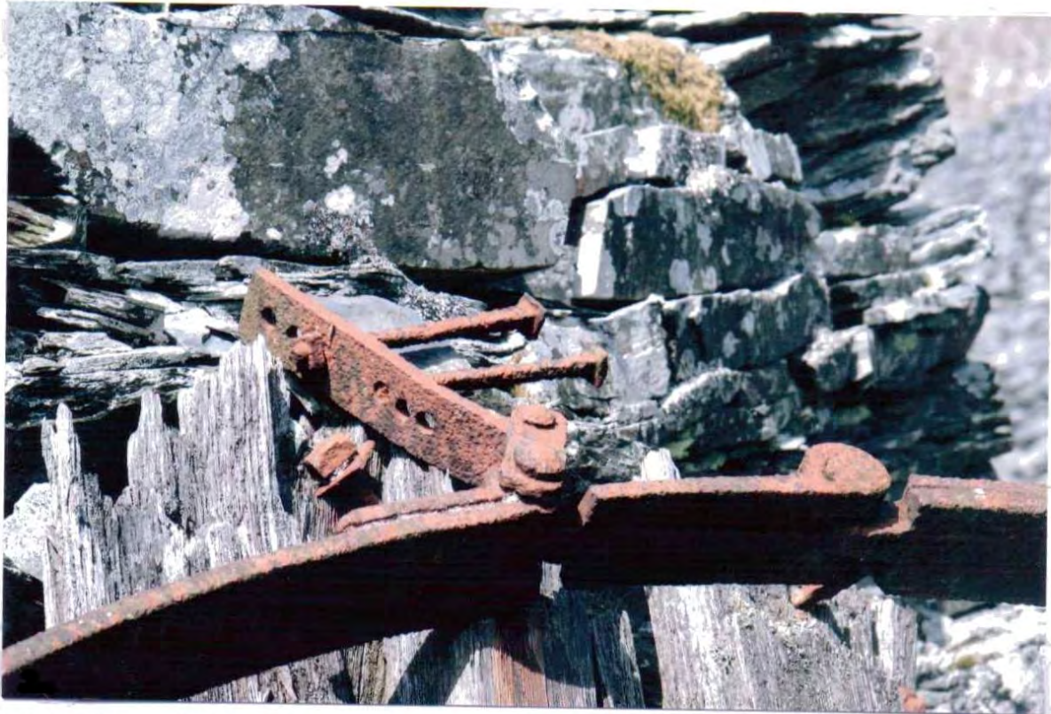
Photo 11. At the rear of the drum, the brake band was jointed and pivoted to a timber member, which has totally disappeared.
