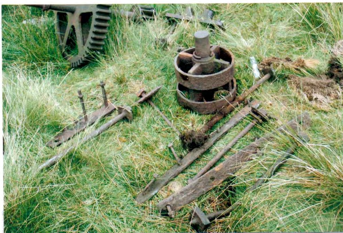
Photo 18. Ironwork found at the summit level of the Cae Abatty Tramway. The holding down bolts and straps indicate that there was a timber structure on the site.
