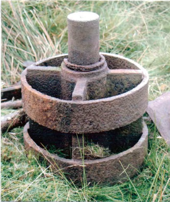
Photo 7. Axle end cap from the winding drum at the Summit of the Cae Abatty Tramway. No recognisable timber remains from the drum or its supporting structure.
