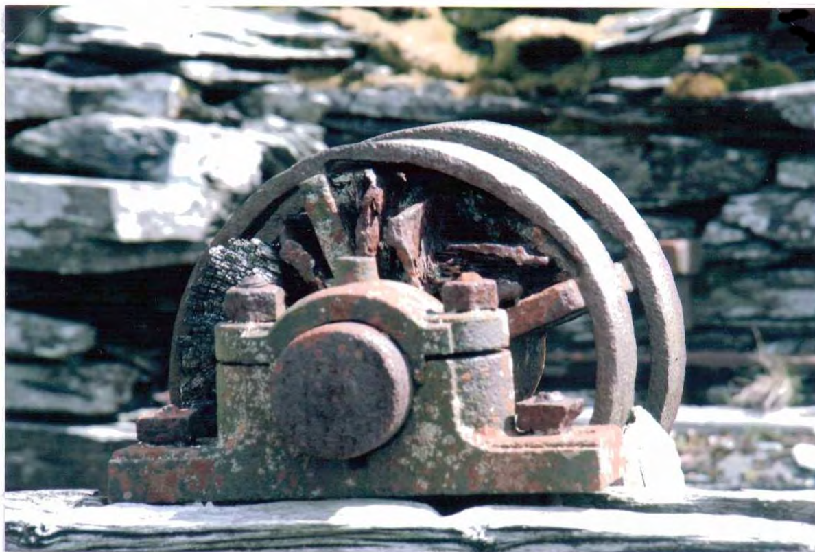
Photo 5. The West axle end cap of the Cae Abatty Quarry Incline Drum, still in place in its bearing block on the drumhouse wall. The remains of the axle within the end cap have rotted away.
