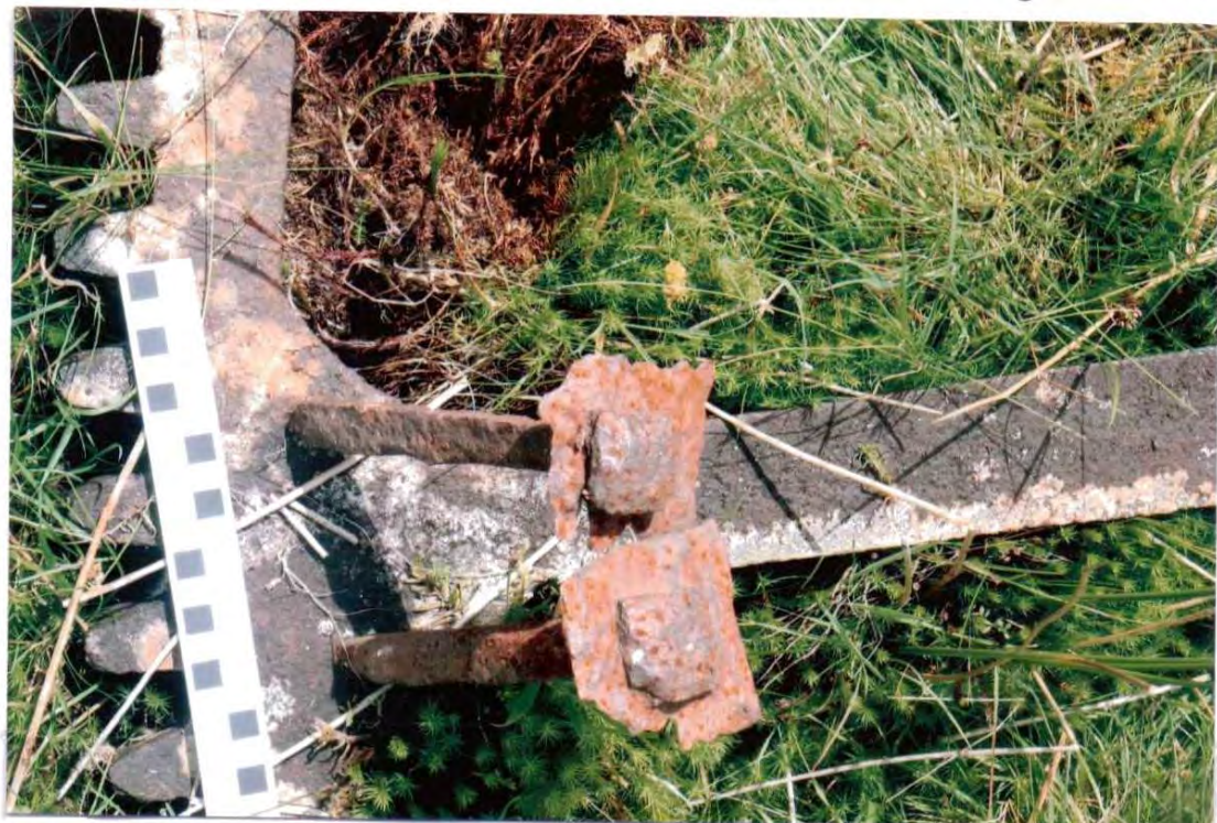
Photo 32. One of two pairs of bolts on the periphery of the large gearwheel. Four pairs of bolts would have fixed it to one spider of the winding drum.
