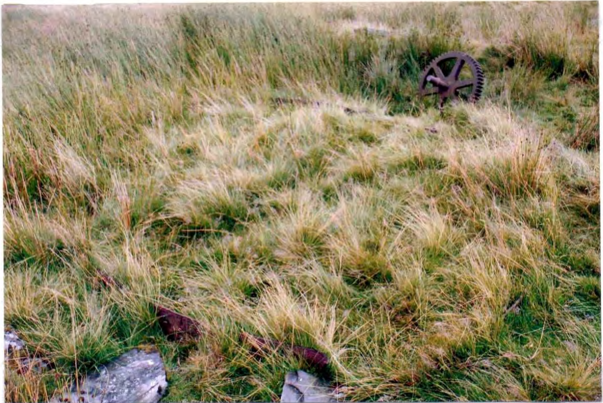
Photo 19. Parts of the brake band and braking surface rim, laid out as a single circle in the grass at the tramway summit
