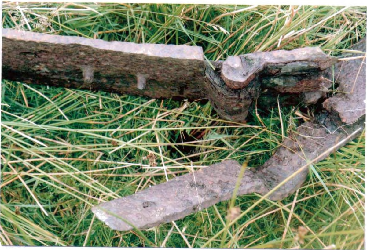
Photo 24. Another of the joints in the brake band has broken, and has been repaired by a strap.
