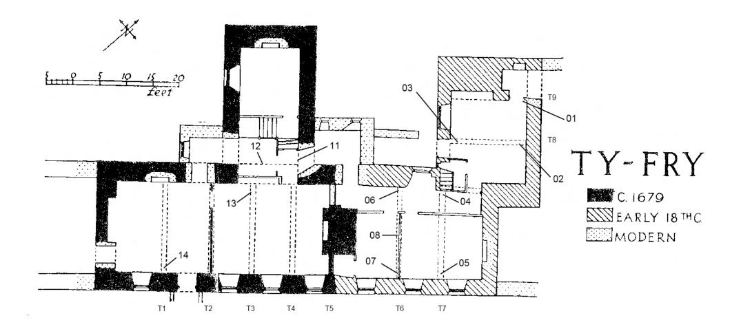
Figure 1: Plan of the property showing the timbers sampled for dendrochronology (adapted from an original in the RCHAMW Inventory 1937)
