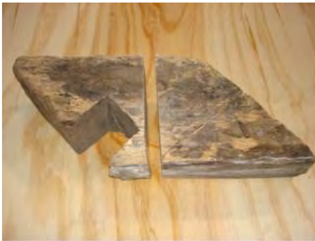
Fig 1a: Timber angg01 showing location of sample slice with II chiselled carpenters' mark
