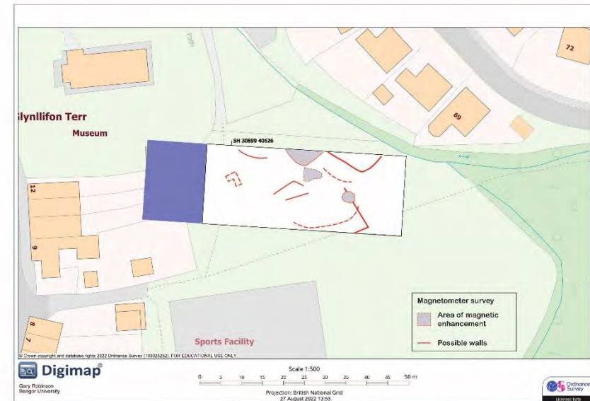
Figure 2: Anomalies observed in the magnetometer data, overlaid for clarity. Prepared by Dr Kate Worthington and Siân Evans, 4 th April 2023. Map taken from Digimap. ( Digimap (edina.ac.uk) )
