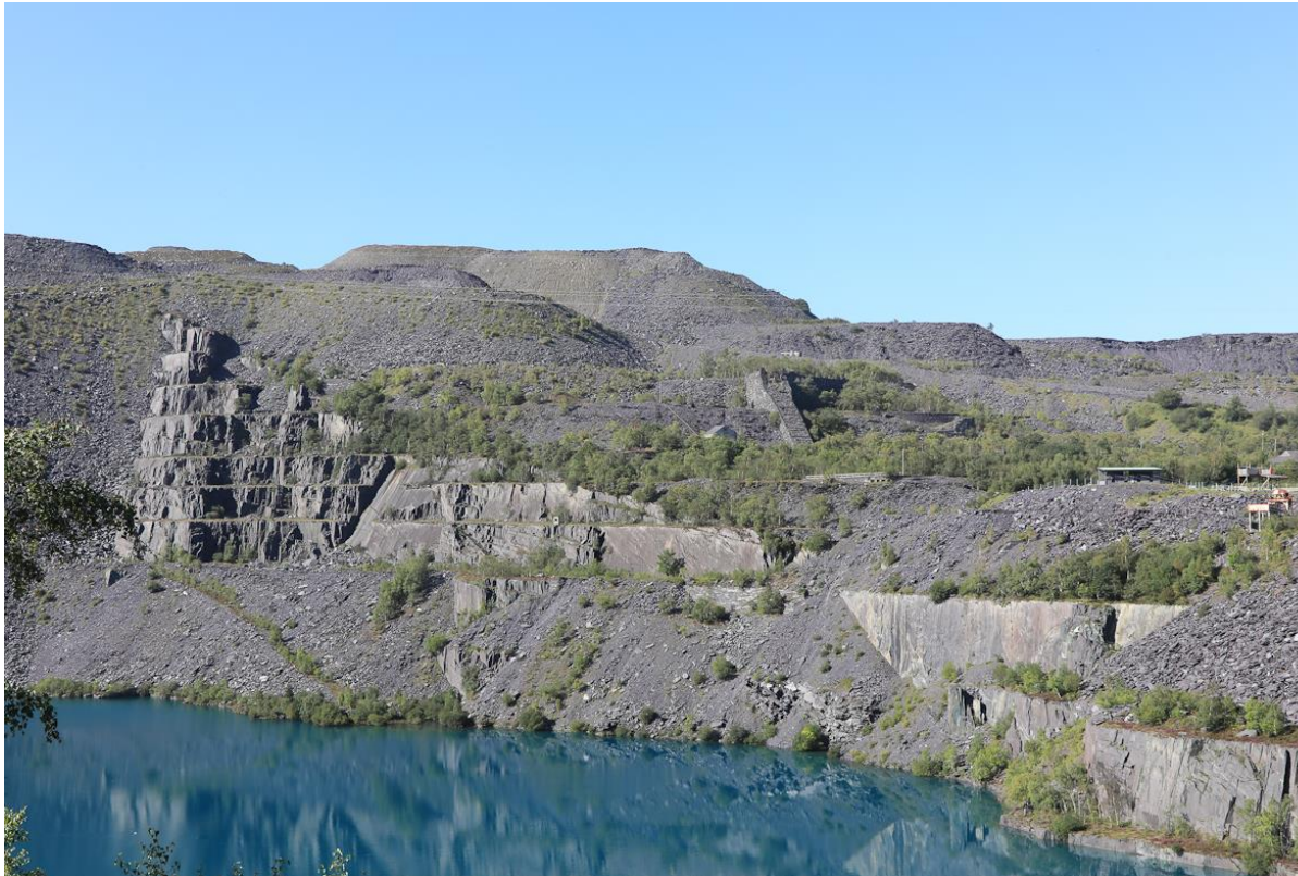
Figure 5: A view looking westward over the 'right side' showing the quarry landscape, including tips of waste rock, stepped galleries and an inclined plane. To the right of the photograph, the 'Princess May' shaft headframe is visible.
