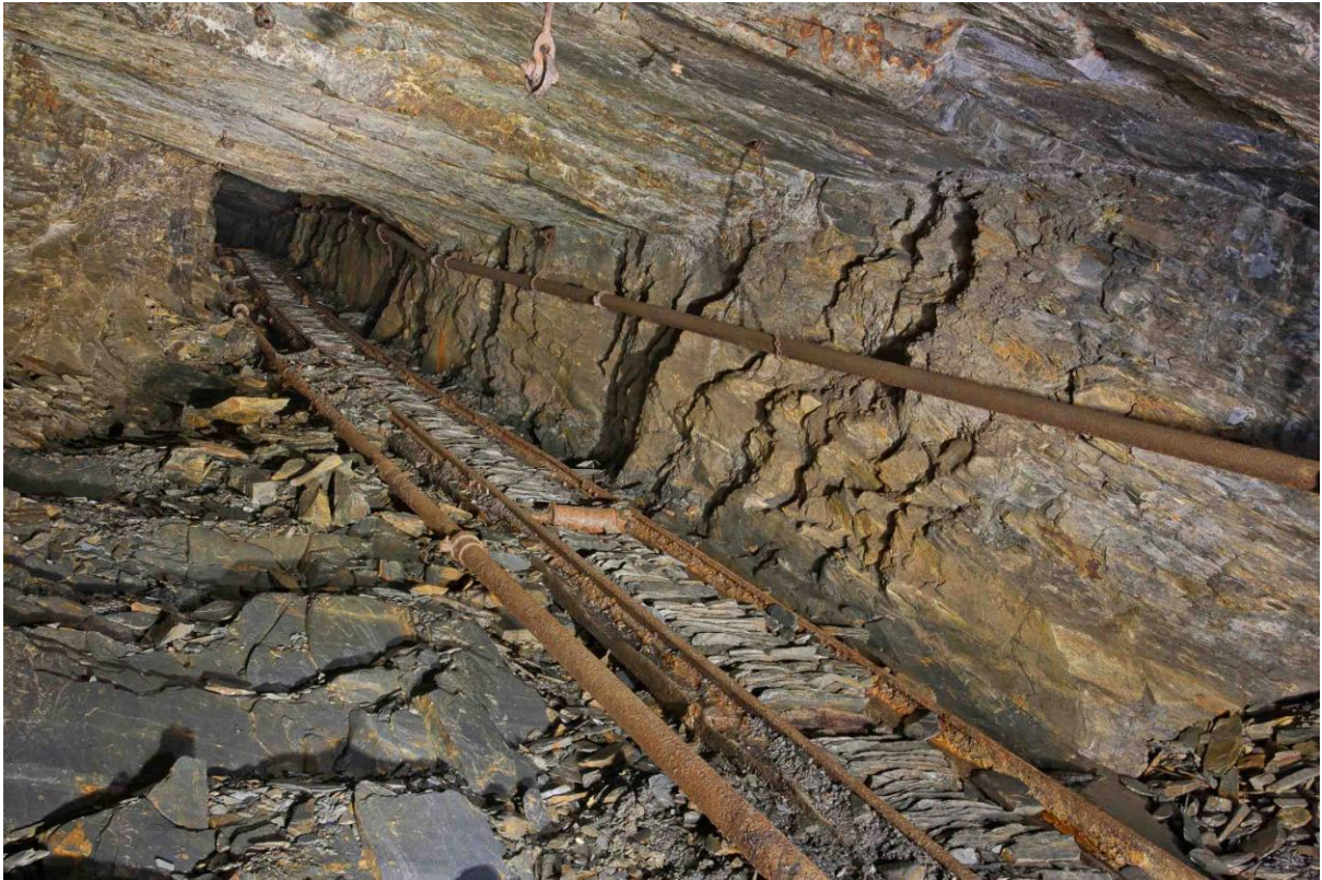
The Back Vein or North Sinc incline in Cwmorthin is unusual in that it is single track and on a variable gradient. NPRN: 546415; PRN: 67489.
