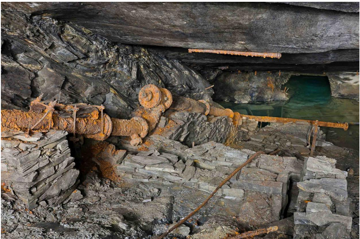
The Ffridd shaft in Llechwedd Slate Quarry connected with the underground workings and enabled a surface water wheel to operate pump rods. Rock-falls have obscured the arrangements here. NPRN: 546431; PRN: 60307.
