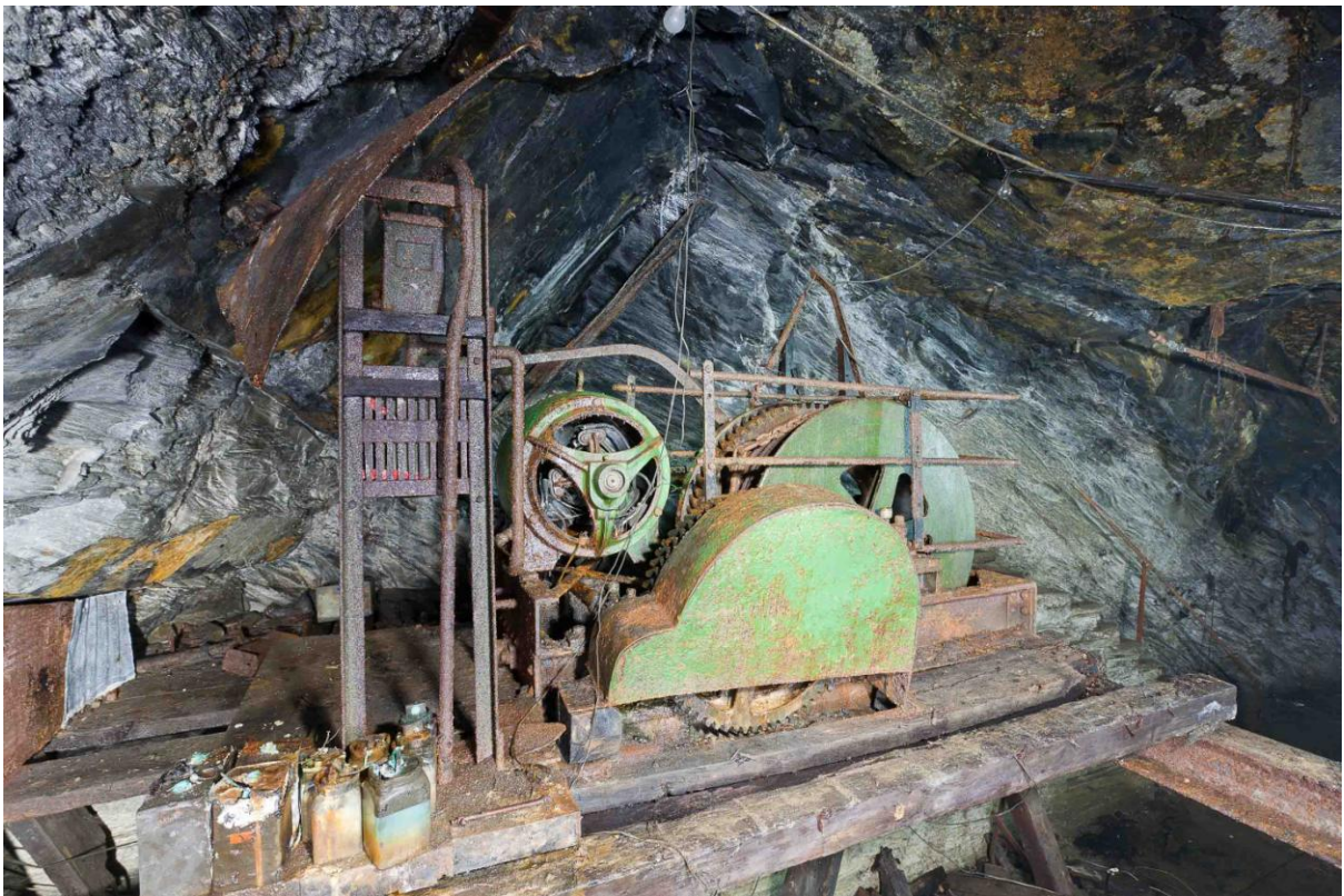
The New Ffridd incline in Llechwedd Slate Quarry retains its state-of-the-art Sandycroft Foundry electric motor and winding drum of 1909. NPRN: 546427; PRN: 67454.
