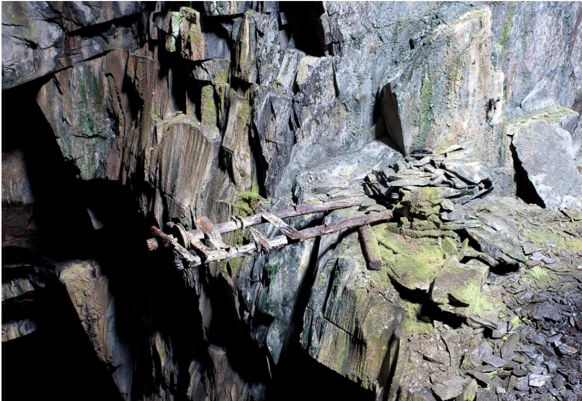
Ceunant Ddu Chamber 1/2 contains a wealth of early/ mid-19 th century artefacts, including this turntree platform. NPRN: 546471; PRN: 67502.
