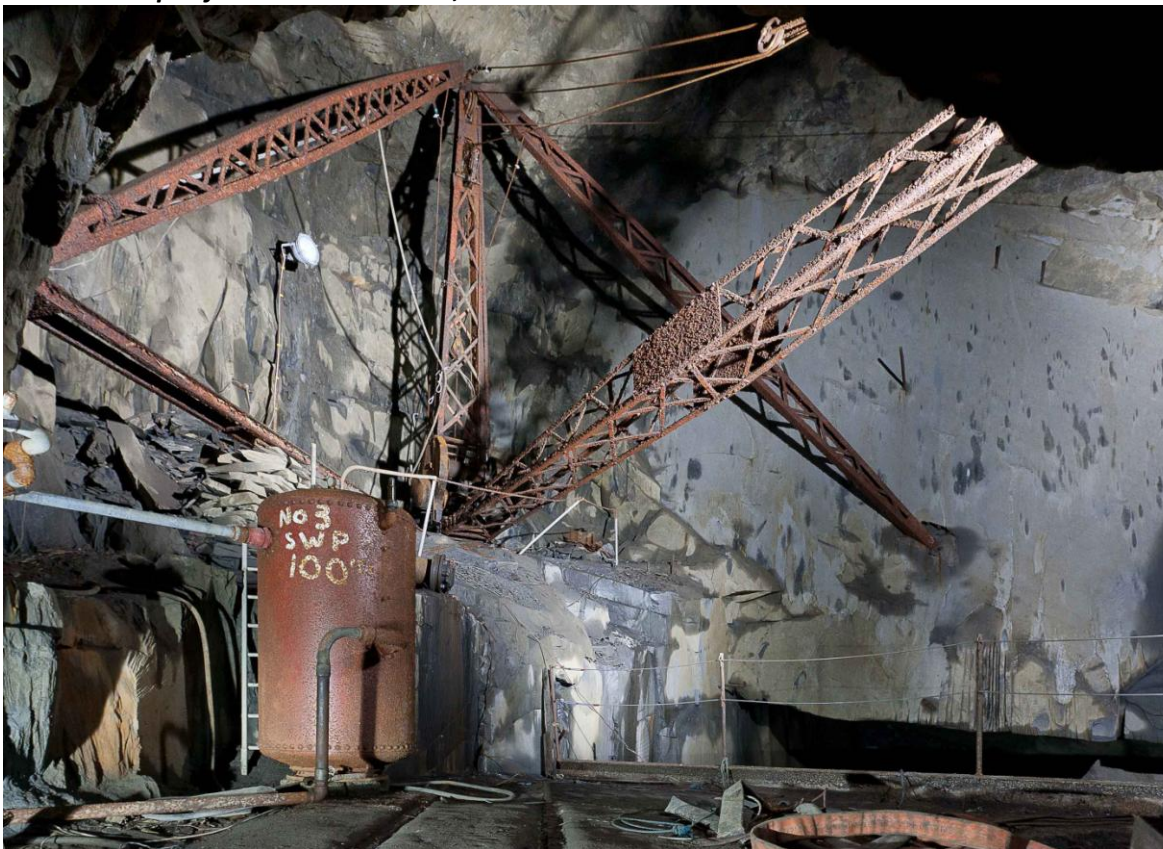
Large-scale late 20 th century engineering at Aberllefenni is represented by this derrick crane in Foel Grochan chamber 5. NPRN: 546485; PRN: 9301.
