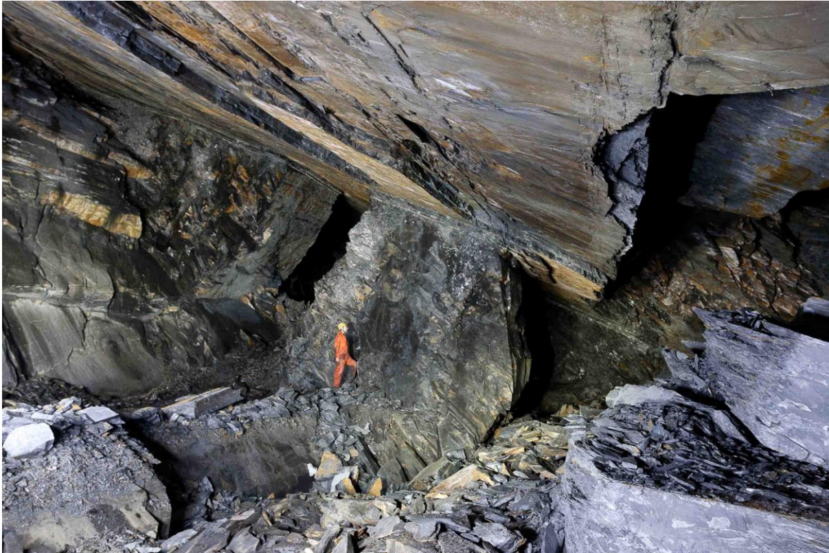
Floor 2 in Maenofferen is the only known location in Gwynedd where the early method of supporting the chamber roof on a free-standing pillar is evident. NPRN: 546447; PRN: 67473.
