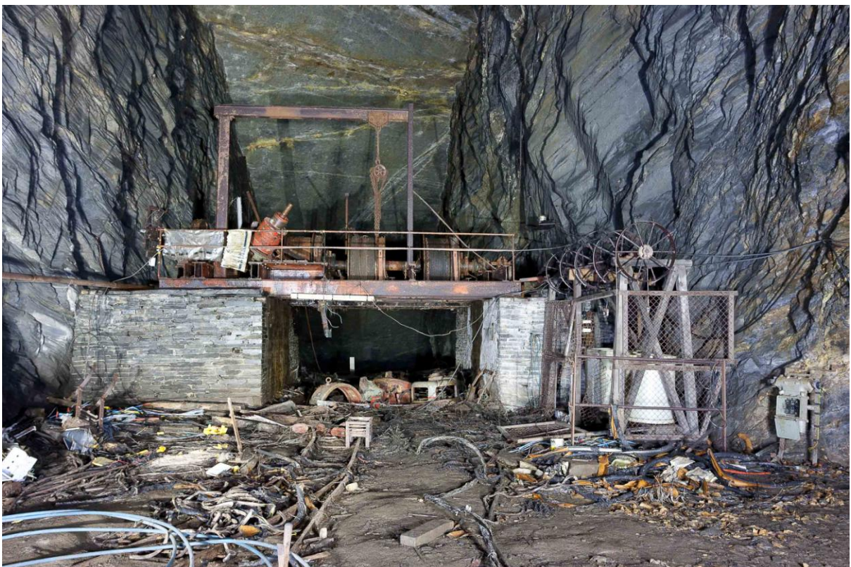
A Peebles motor with double reduction gearing and the three drums provided the winding gear of the B31 incline in Maenofferen. It has been vandalised. NPRN: 546441; PRN: 67467.
