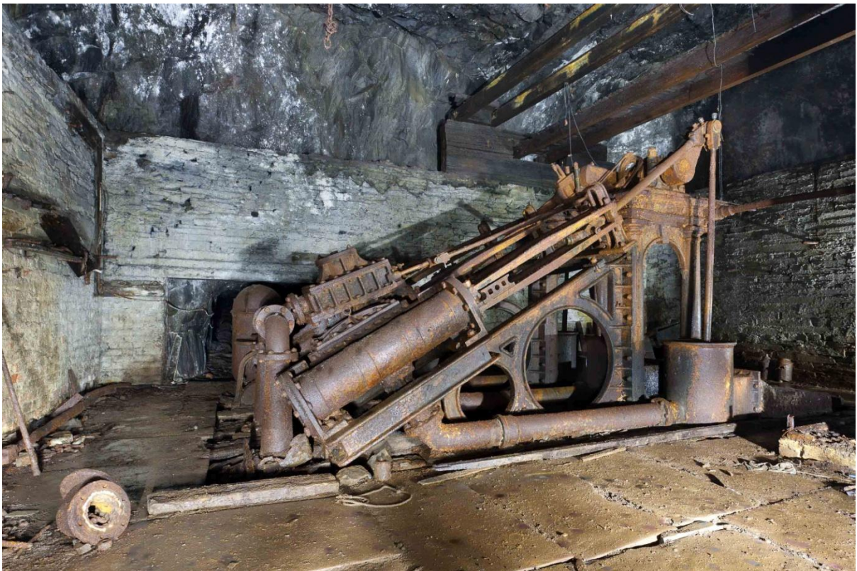
The surviving hydraulic engine in the pump chamber, showing the vertical bucket pumps. Beyond the cylinders, the surge vessel and the tunnel to the 'Lord' water-balance shaft are evident. NPRN: 546403; PRN: 67521.
