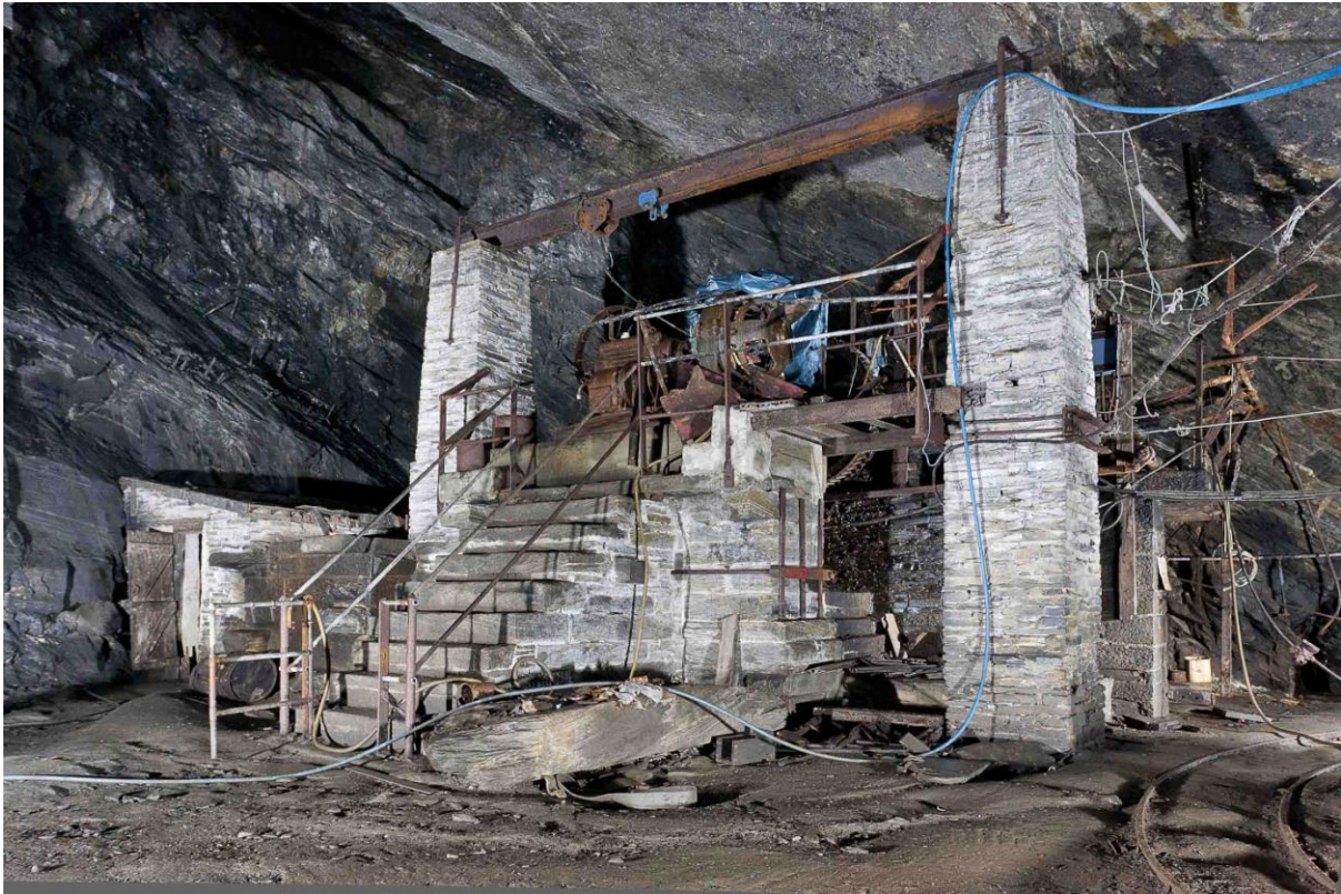
The B8 incline winding gear survives largely intact. NPRN: 546443; PRN: 67469.
