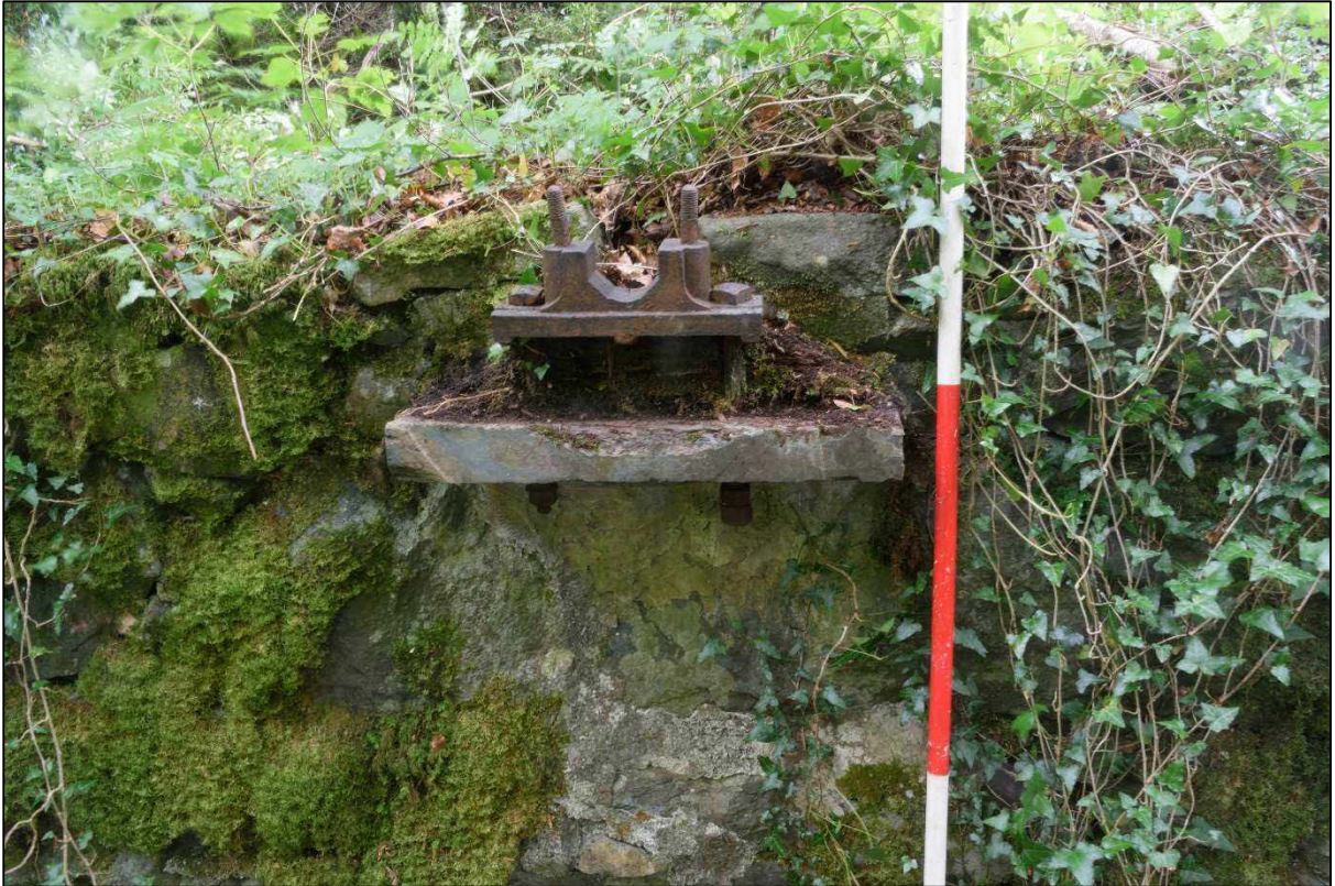
Plate 7: Bearing for the wheel
