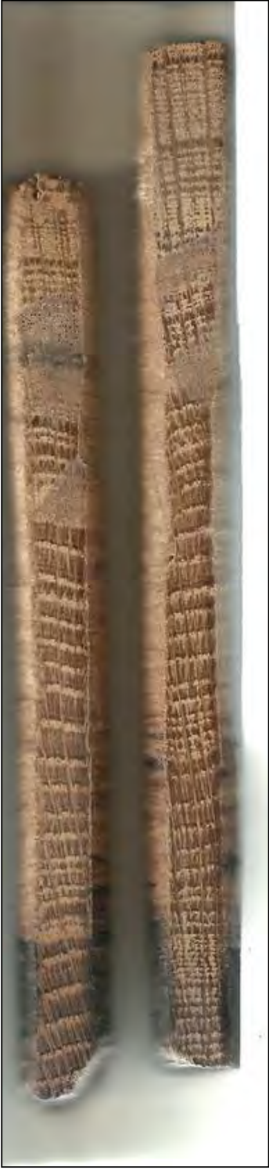
Figure 4: Scan of cores pmr01 and pmr02 , showing bands of narrow rings. Some areas have been cut with a scalpel to aid in distinguishing ring boundaries.
