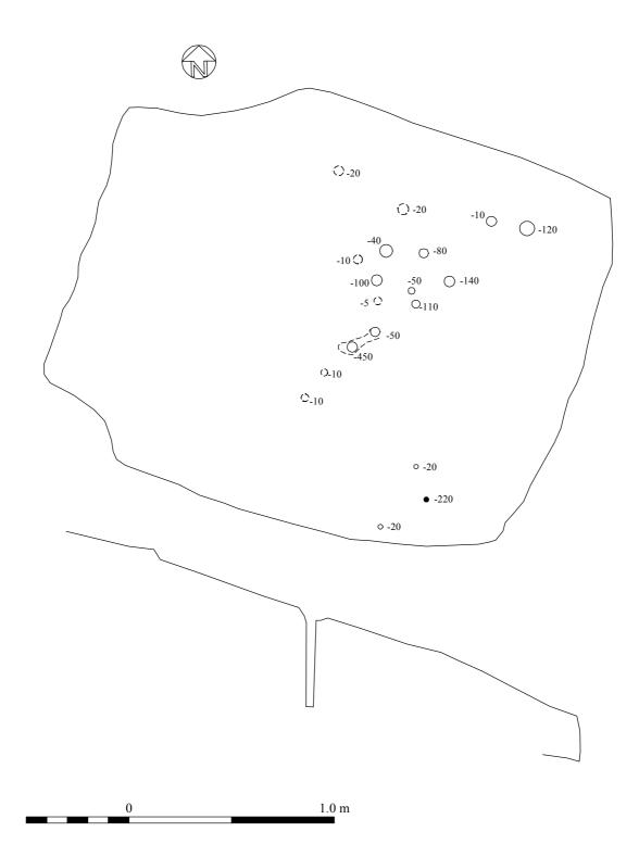
Figure 20: Rock Cannon associated with Tai'r Frest Scale 1:20 Hole depths shown in millimetres
