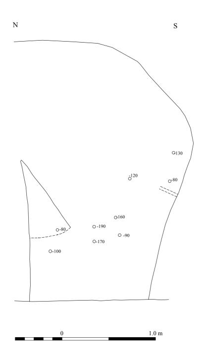
Figure 18: Rock Cannon Associated with Adit PRN 14688 Scale 1:20 Hole depths shown in millimetres
