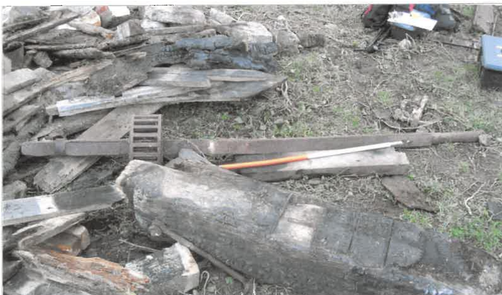
Plate 22: Quant with stone nut (slipped to bottom)
