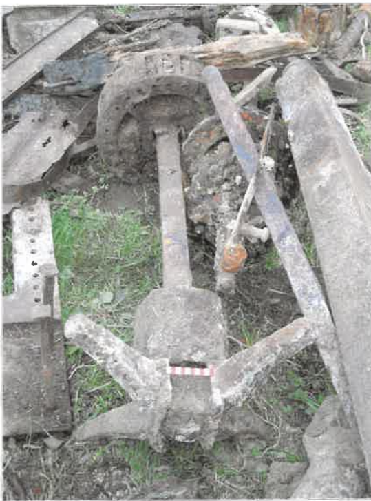
Plate 24: Bridge tree with integral quant and wheel nut
