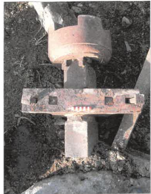
Plate 20: Dog clutch and bearing (on main drive shaft)
