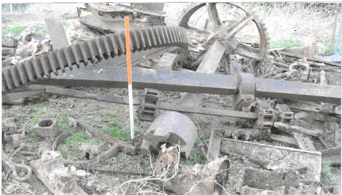
Plate 17: Wallower, drive shaft, lay shaft and spur wheel
