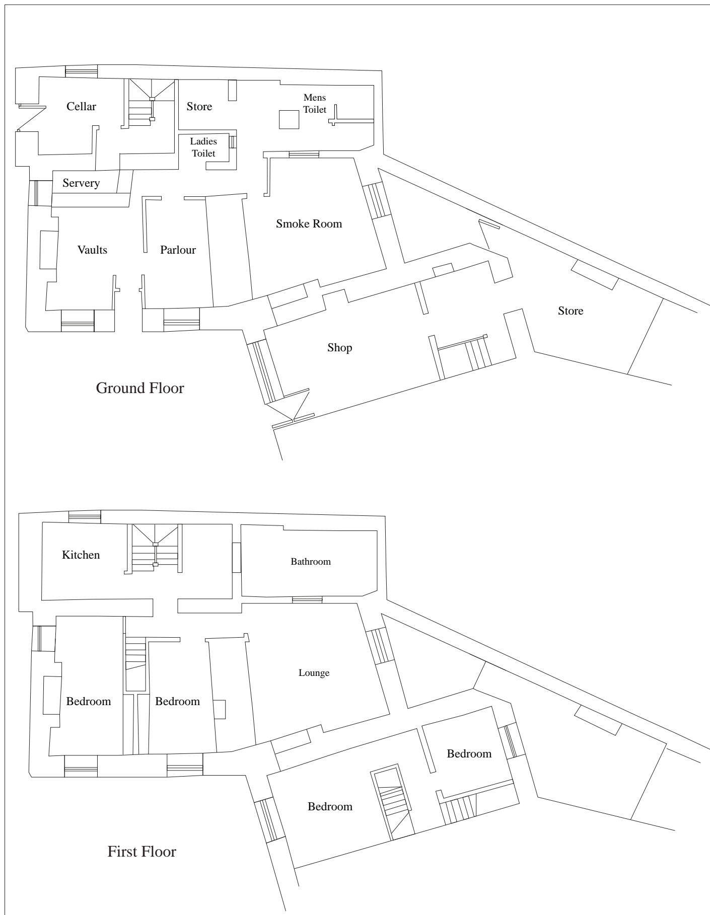
Figure 29. Caernarfon Castle Public House Existing Floor Floor Plans in 1976 Copied From 1970's Originals. Scale Given 8'0" to 1 Inch
