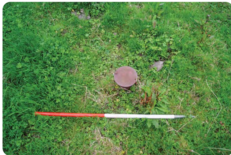
Plate 8. Upright Metal Pipe Presumed to be for Measuring Water Table in Field 1.
