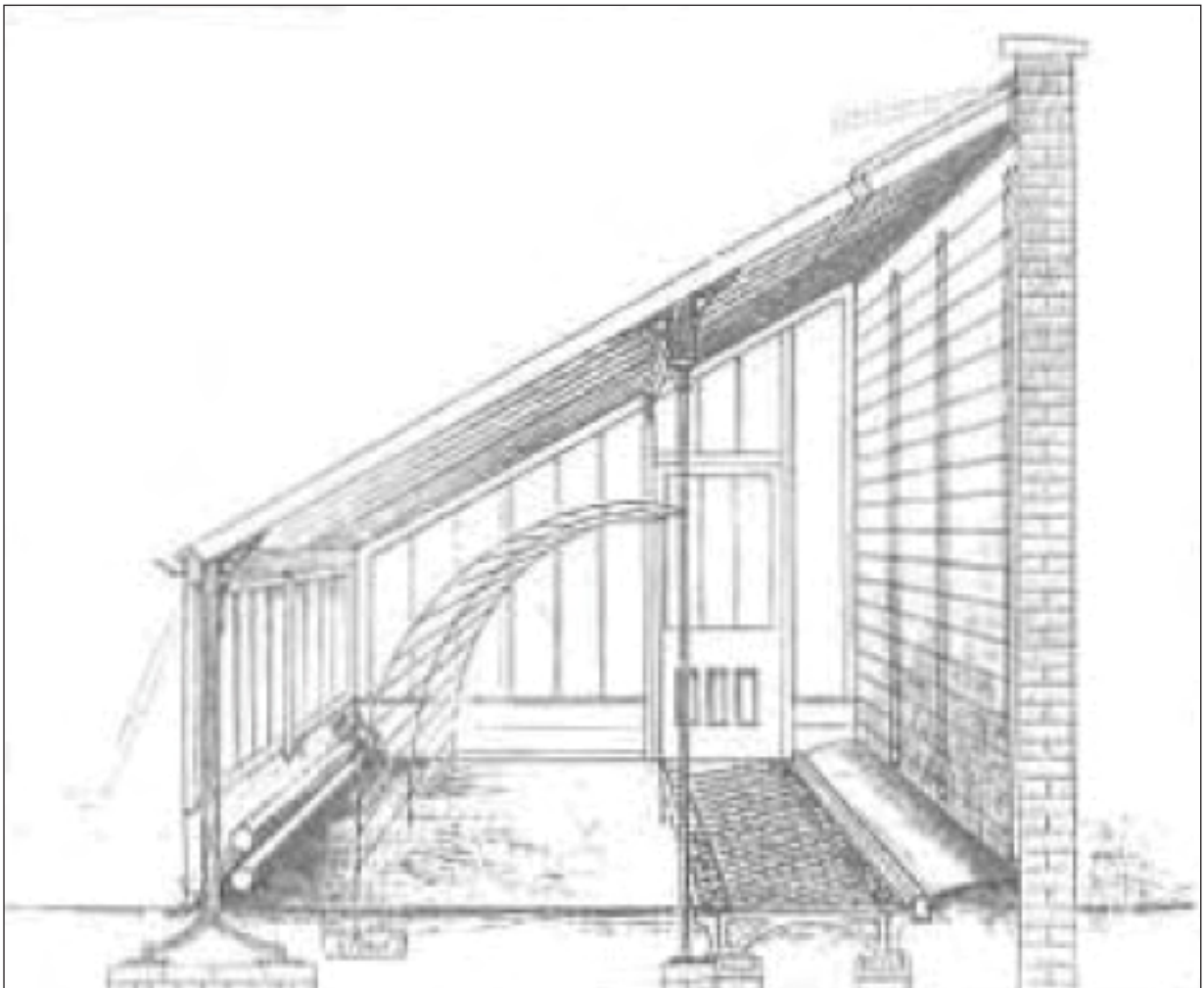
Plate 73. Cross-section Through Lean-To Peach House Similar to that at Benarth Hall. Source Fosters & Pearson 1909 Sales Catalogue (Page 50)
