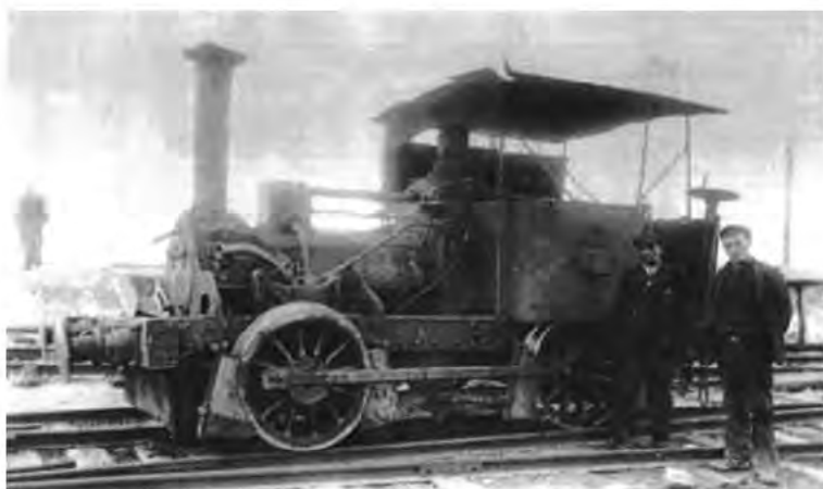
a) Early locomotive used on breakwater railway line. 7ft gauge Longridge 0-4-OWT at Holyhead on 5 March 1912.
