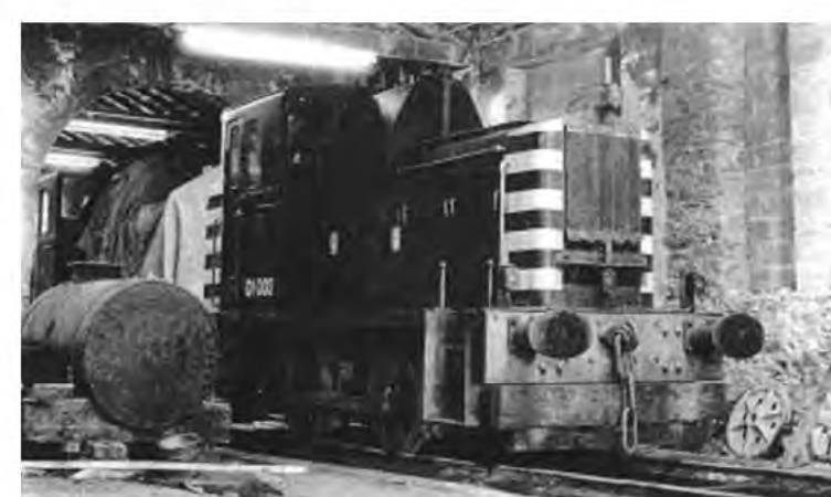
c) Early locomotive used on breakwater railway line. Class 01 Barclay diesel in engine shed 1979
