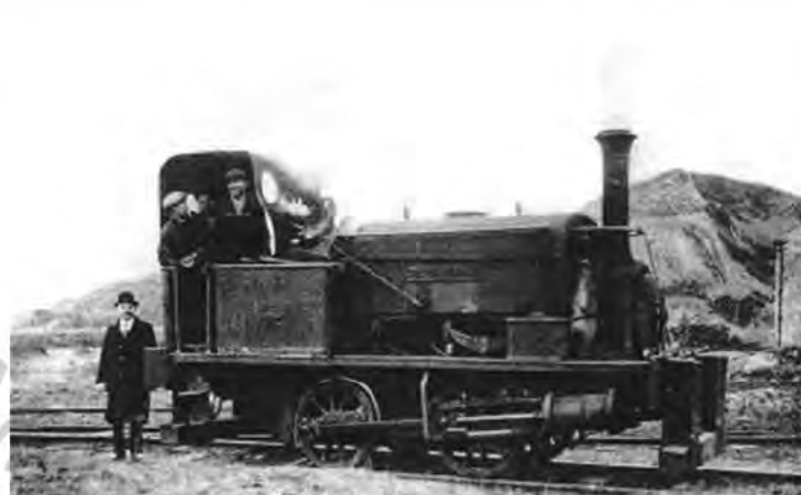
b) Early locomotive used on breakwater railway line. Manning Wardle Manning Wardle 0-4-OST CROWHURST engine on Breakwater c. 1900
