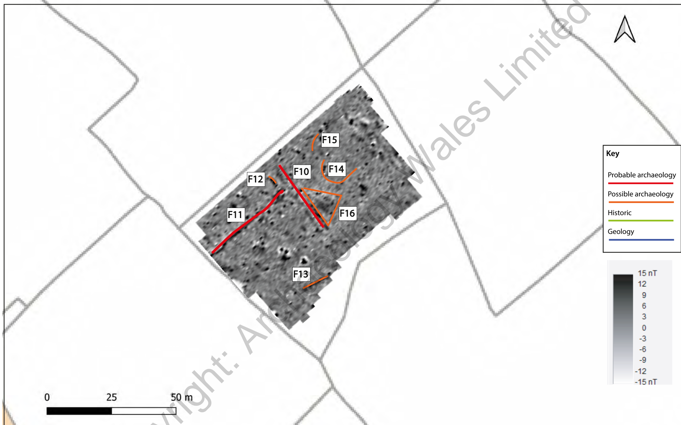
Figure 7. Field 3 - Greyscale plot of processed data clipped to \pm 15
