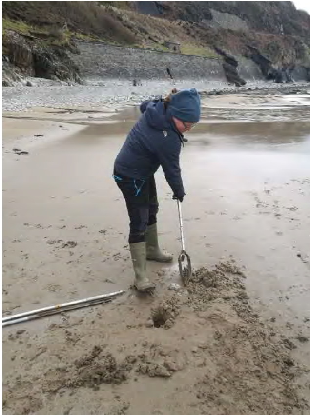
Plate 3: Edelman auger in use for initial spot samples
