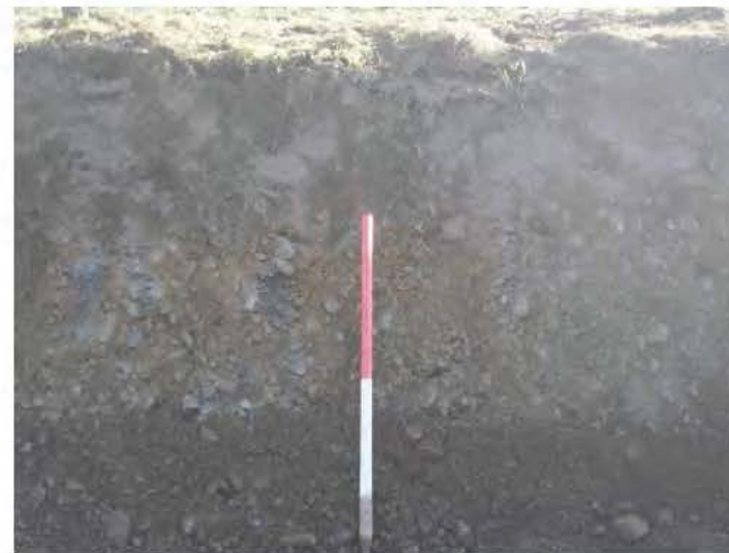
Photo 6. Section 2. Detailed shot of section showing depth of topsoil and 2 bands of natural gravel. 1m scale, Facing South.
