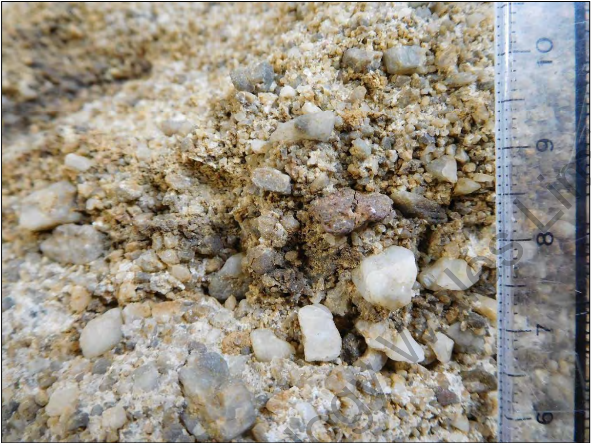
Figure. 4: Specimen LMCE / 17 / EX (1041) 024 – weathered jasper (centre) and protruding quartz grains in weak carbonate cement
