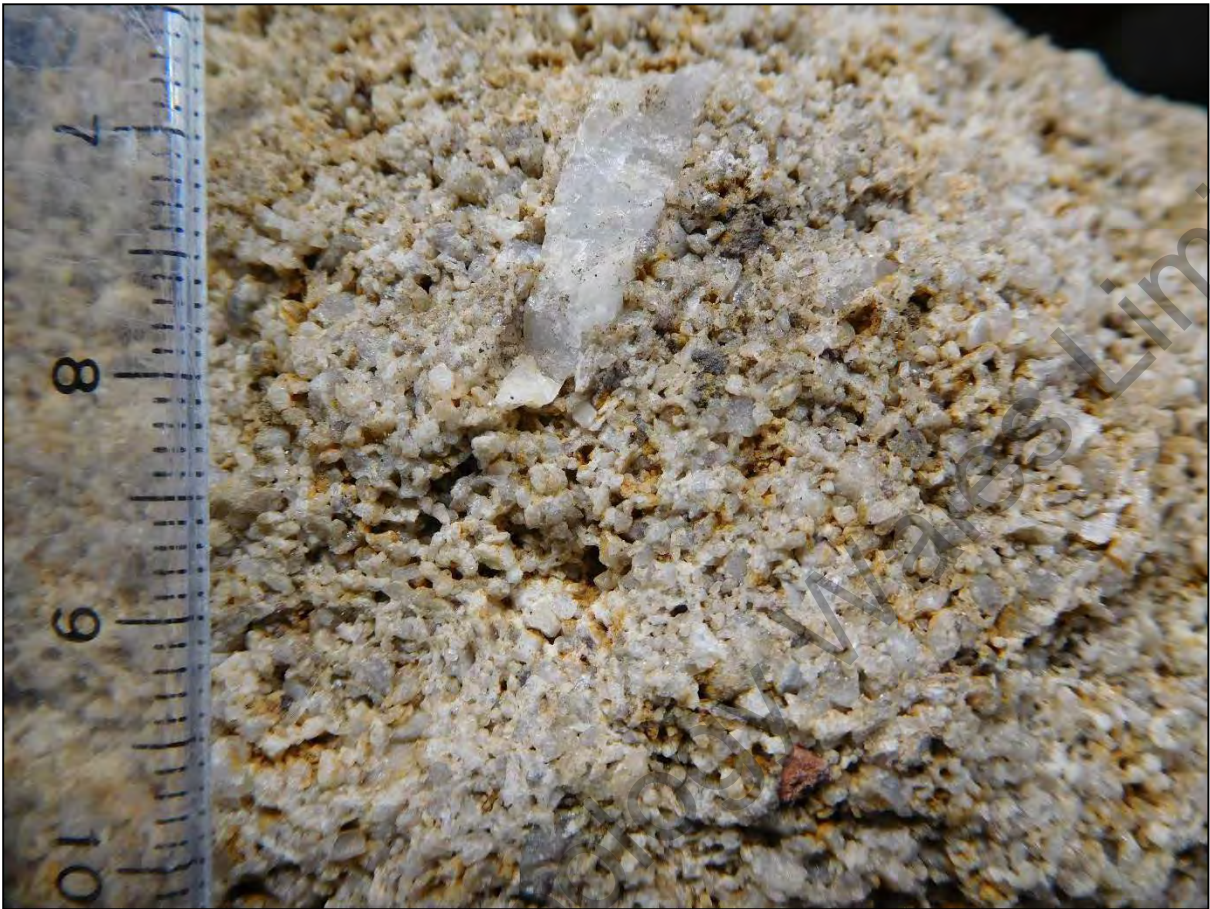
Figure. 1: Specimen LMCE / 17 / Ex SF. 001 (1002) - Granular texture of sandstone with large sub-rounded quartz pebble (centre top) and rare red-coloured lithic grain (bottom right)
