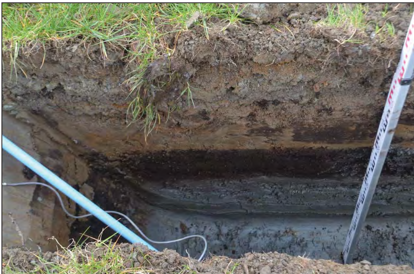
Plate 24: TP 123 - Section view of TP 123 showing peat and alluvial clay layers close-up; scale not used; view from NNE (archive reference: E49206_024).
