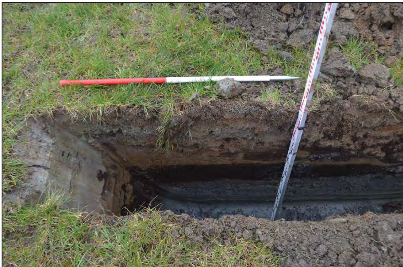
Plate 23: TP 123 - Section view of TP 123 showing peat and alluvial clay layers; scale 1x1m; view from NNE (archive reference: E49206_023).
