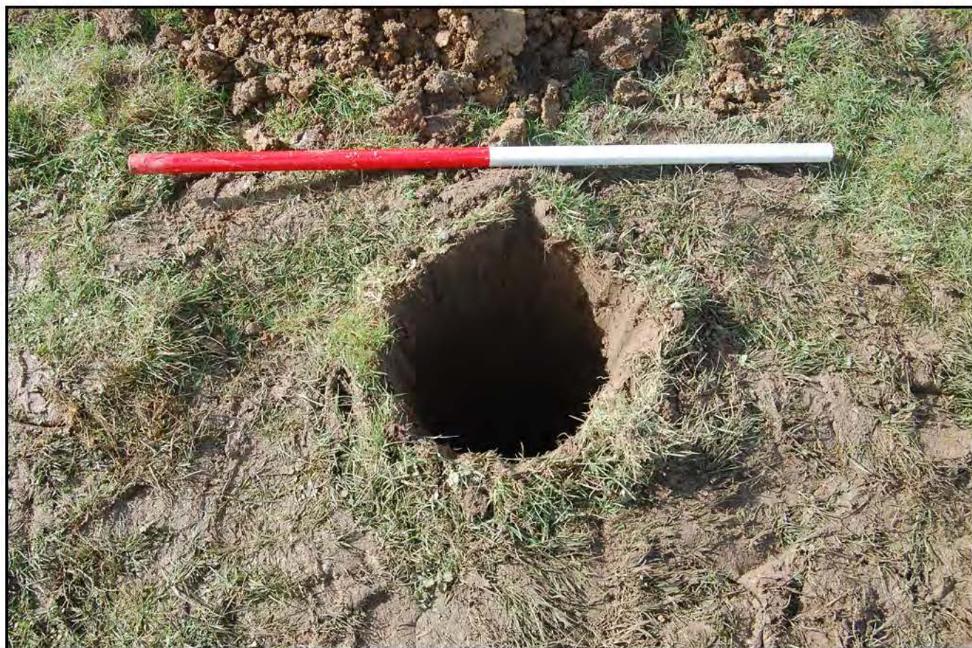
Plate 03: An example of a hand-excavated bore hole inspection pit (BH 521 within F1) (Scale 1.0m).
