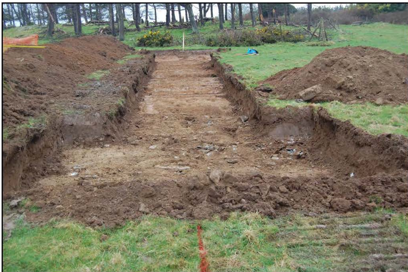
Plate 07: An example of a small Seismic Hazard Observation Trench (OT604B within F56).
