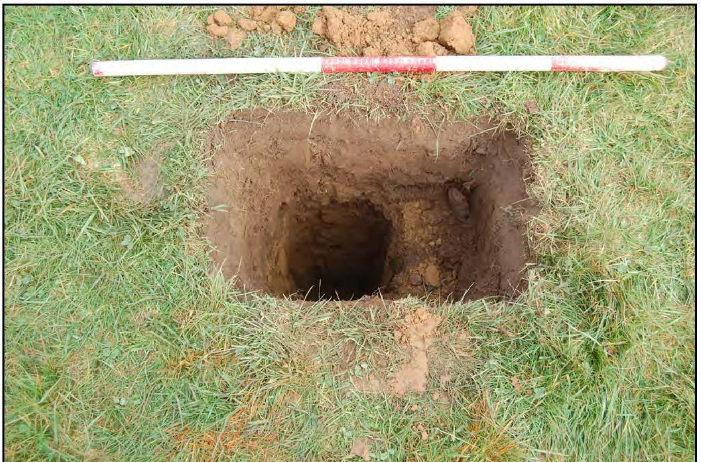
Plate 06: An example of a hand-excavated test pit targeting a geophysics anomaly (TP-76A within F56) (Scale 1.0m).
