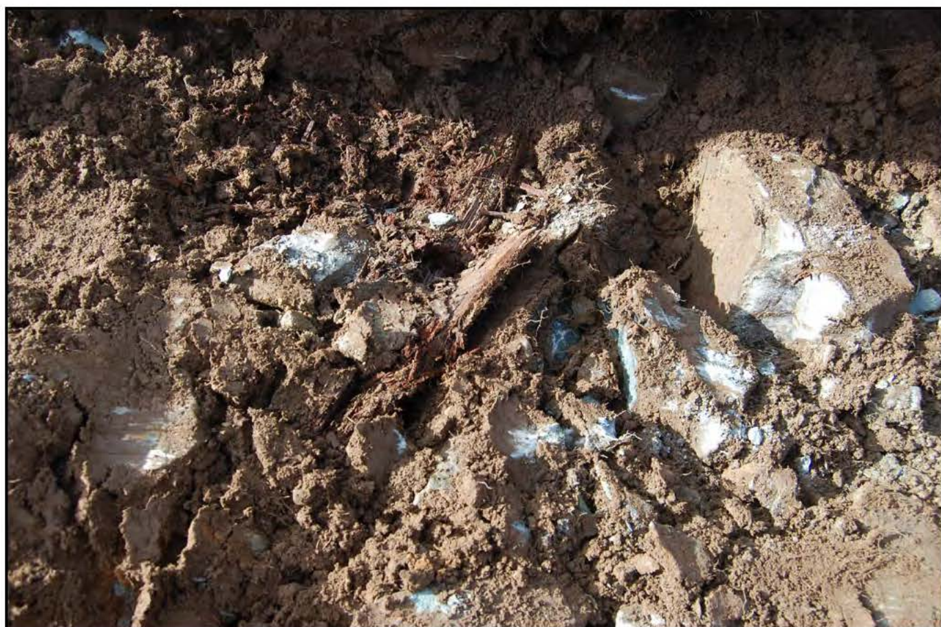
Plate 24: A close up shot of the disturbed area in F1, observed in the haul road trench. The made ground contained frequent boulders and waste material including wood and metal.
