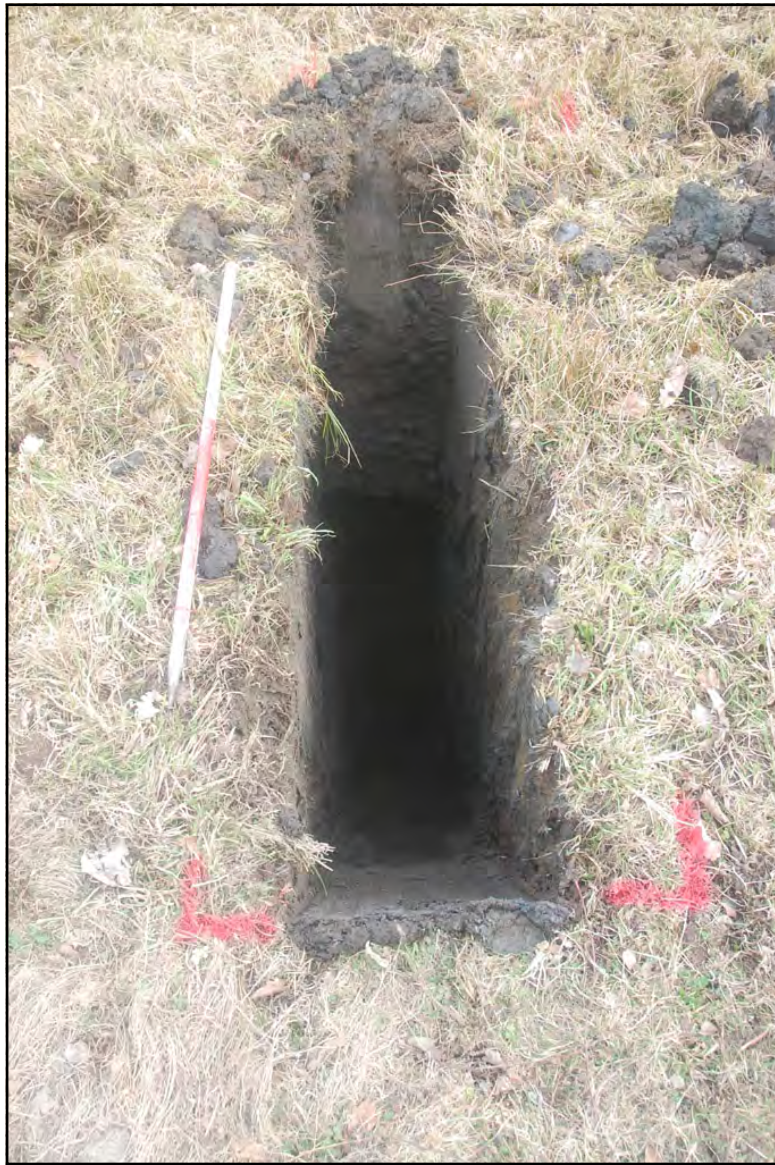
Plate 05 - test pit 05 post-excitation, Similar to test pit 01, peat-rich organic deposits were identified @0.55m below ground level, continuing towards the limit of excavation where the deposit became clay-rich
