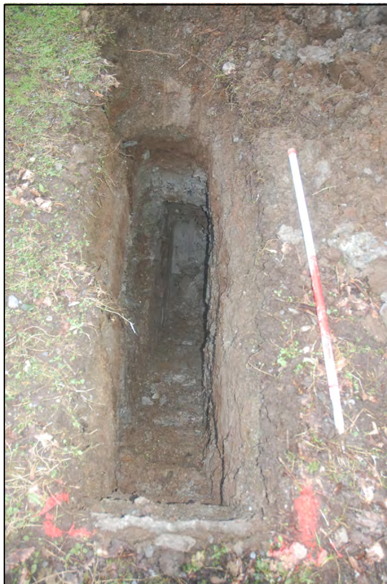
Plate 08 - test pit 04: detail of limit of excavation. The organic-rich deposits and the shale-rich deposit at the base of the test pit (3.00m below ground level), are visible
