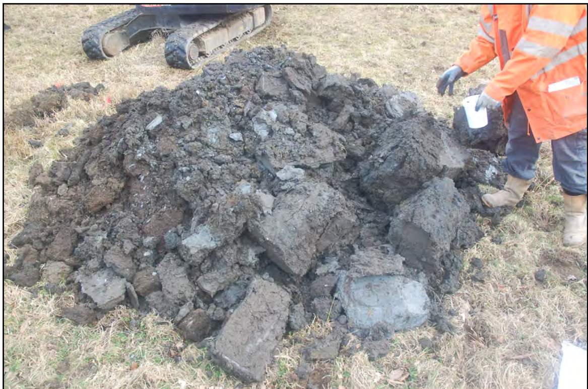
Plate 06 - test pit 05 spoil heap detailing upcast material, including the peat-rich organic deposits also identified in test pit 01 (located c.190.0m to the south).
