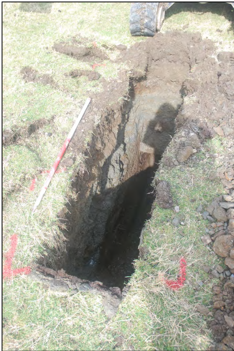
Plate 03 - test pit 01: exposed section on completion. A 0.40m thick layer of silt-sand, peat-rich with frequent organics was identified @1.00m below ground level
