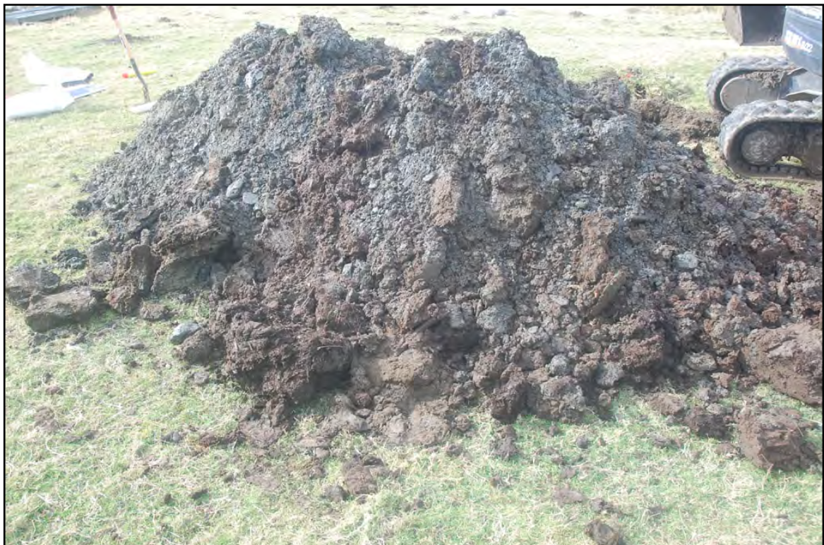
Plate 04 - deposit located beneath the peat-rich layer that continued to limit of excavation (3.00m below ground level)
