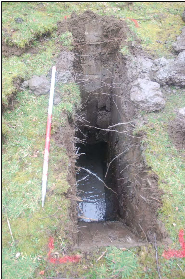
Plate 10 - test pit 10 on completion, detailing limit of excavation and water ingress @1.50m below ground level
