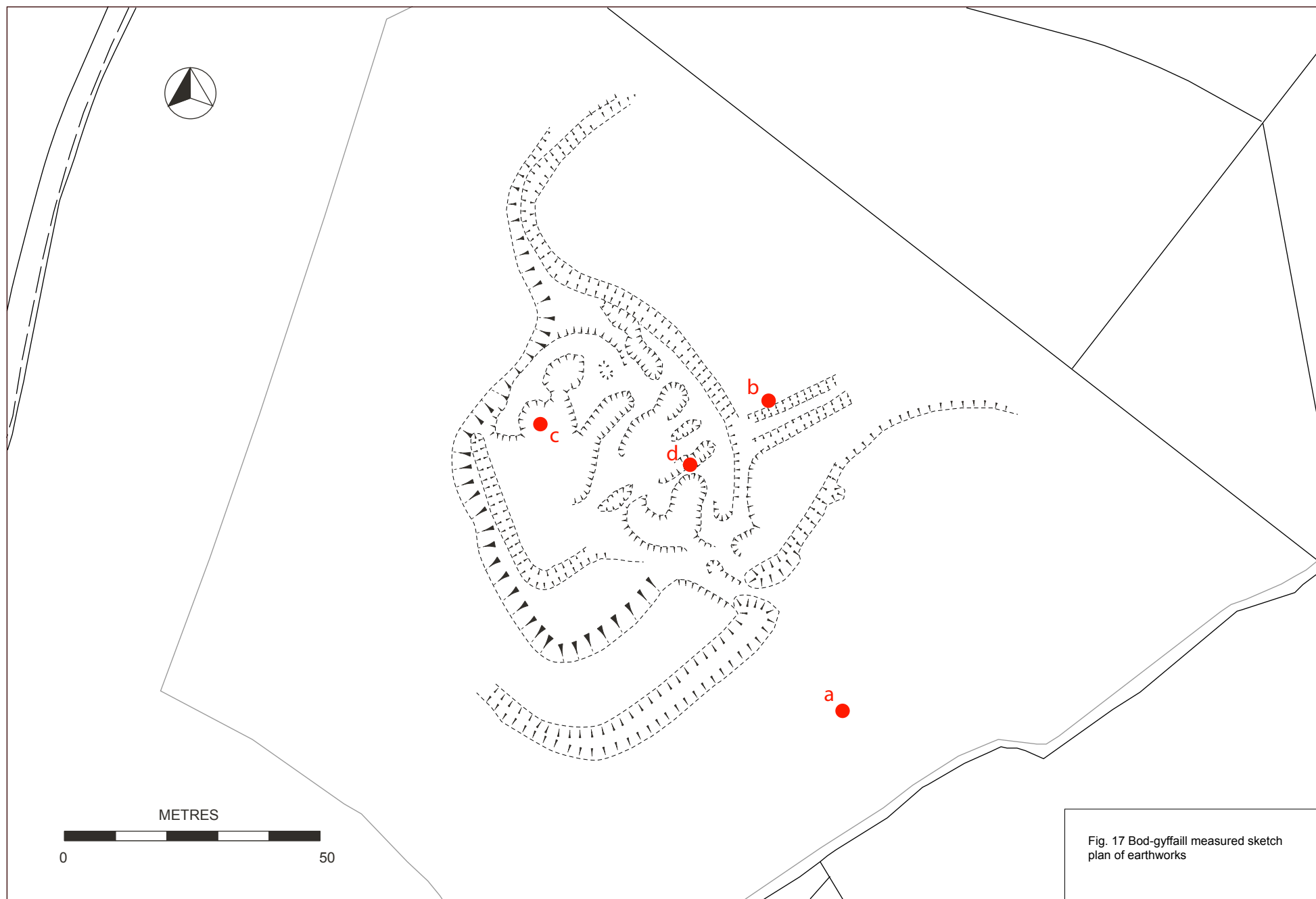
Fig. 17 Bod-gyfaill, Llanfaelog. Measured sketch plan of earthworks and location of soil test pits (a-d)
