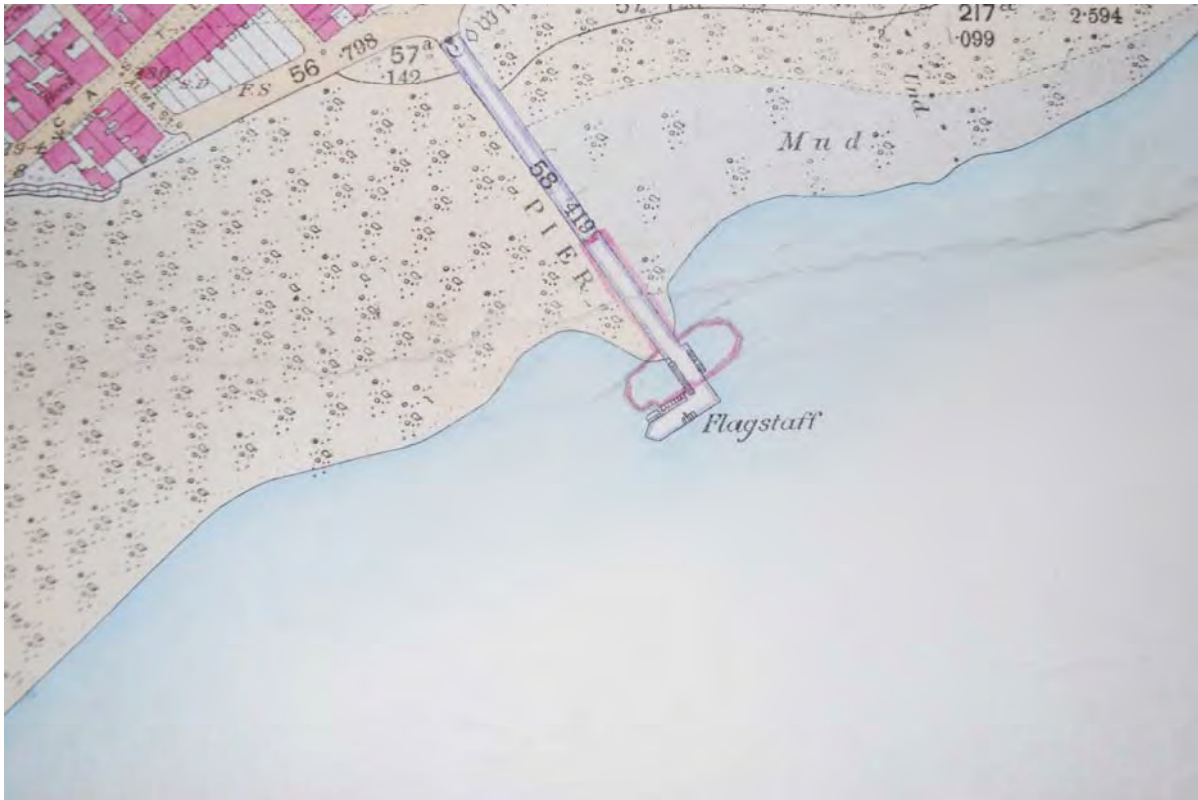
Fig. 7 Extract from 1 st edition 25 inch Ordnance Survey map of 1889. Sheet Caernarvonshire VII.5, annotated with proposed alterations to pier head and creation of 'T' shaped pier head. Dated to approximately 1895.
