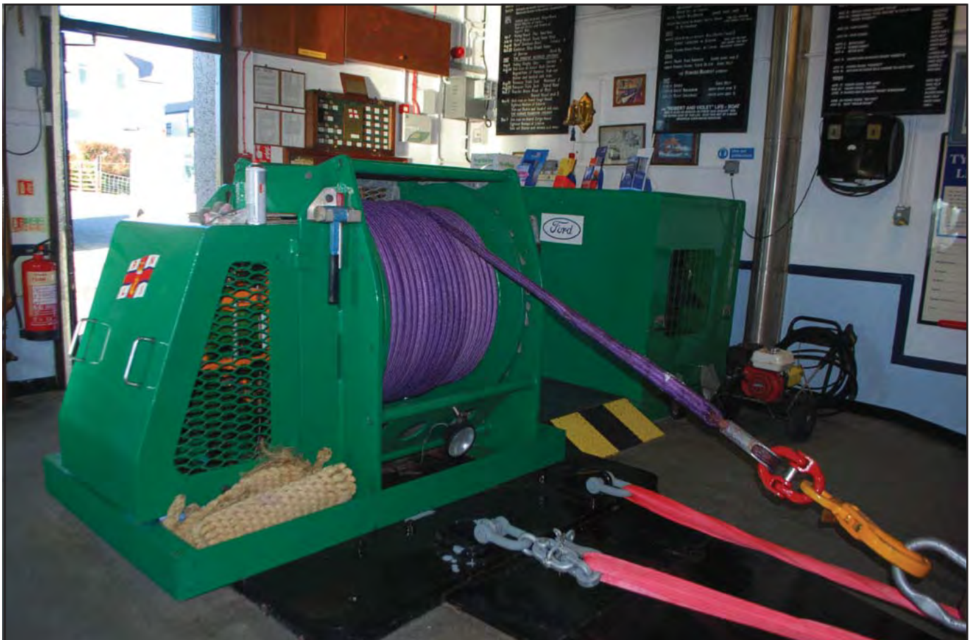
Plate 12 – Hydraulic winding gear within lifeboat house
