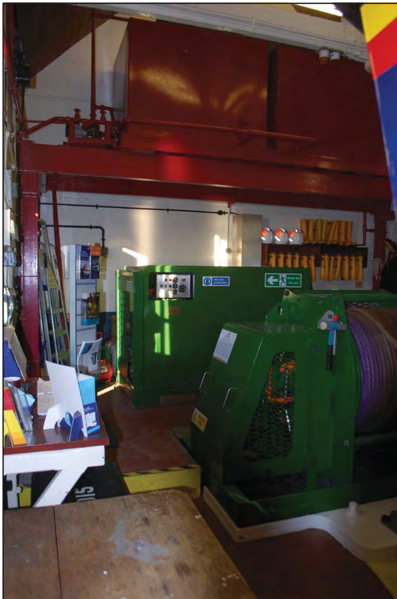
Plate 14 – Hydraulic winding gear and generator
