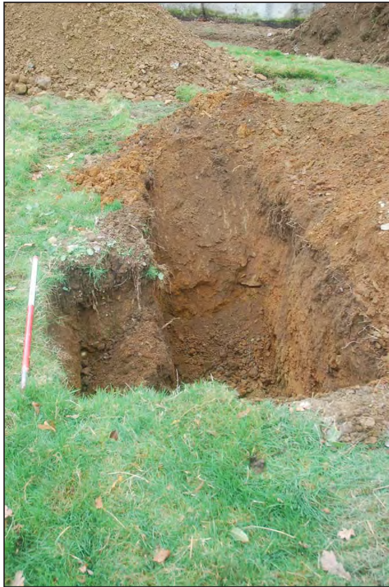
Plate 06: working shot of soakaway detailing exposed sections and stratigraphy. The topsoil was extant to a depth of 0.26m followed by an orange clay-silt; followed by a mid-brown gravel-clay to limit of excavation (ranging pole: 1.0m)
