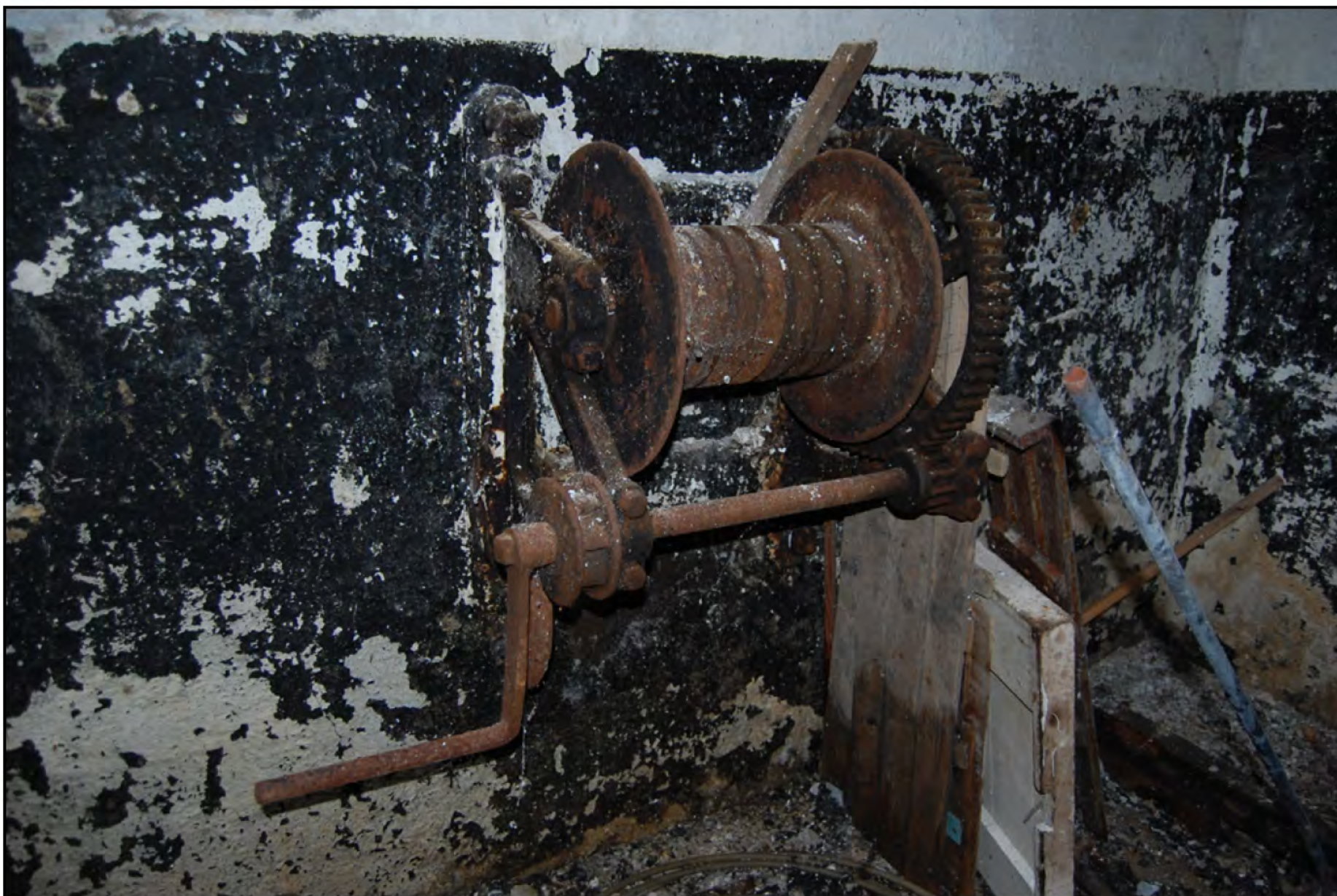
Plate 60: YARD 6 (PRN 30474): Building 08 (PRN 30476) (internal): detail of a large metal hand winch set on the NE wall
