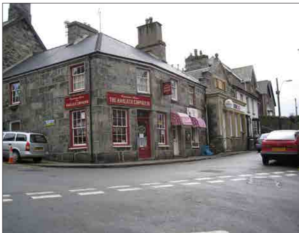
Plate 23. Early 19th century developments in the square were built to a more polite style using thin masonry slabs applied to a rubble wall to produce an ashlar finish.
