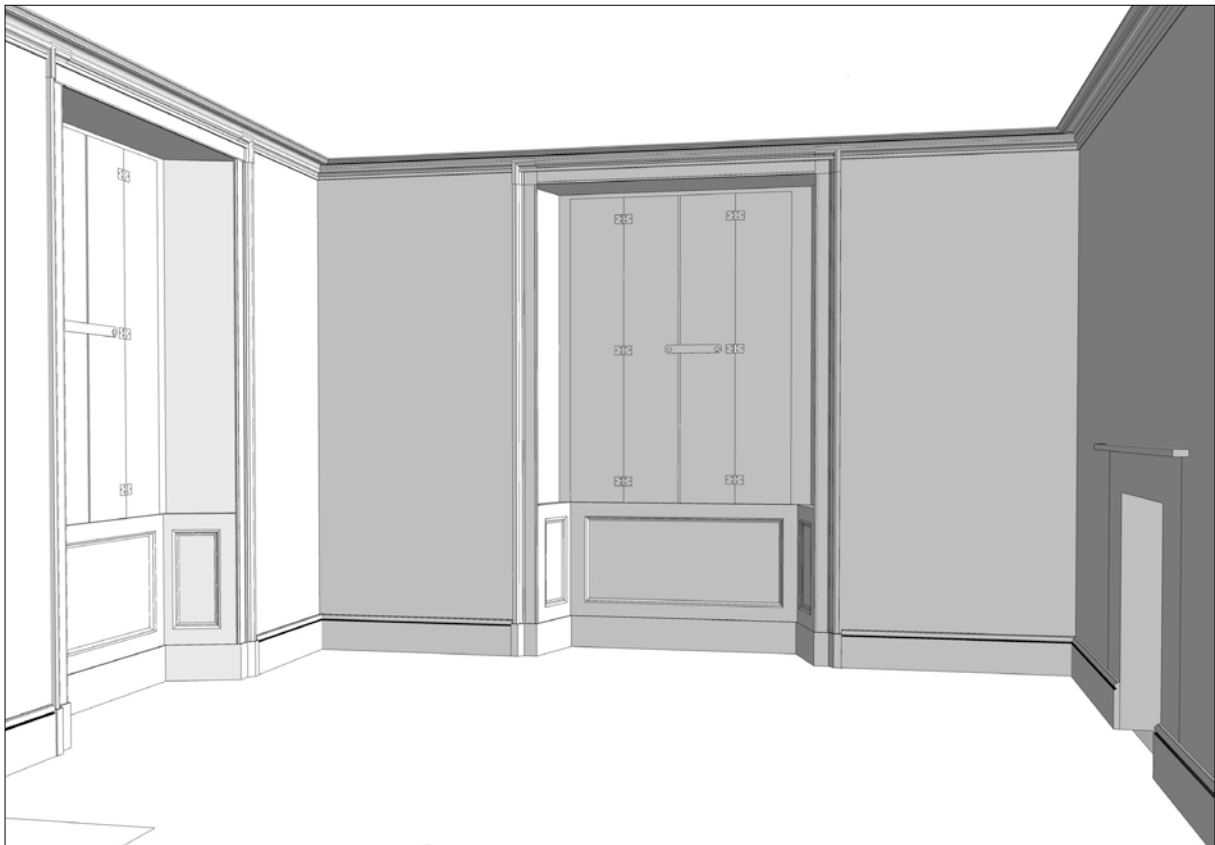
Fig. 44. South office, south room - ground floor, showing shuttered windows, architraves, cornice and fireplace in west wall
