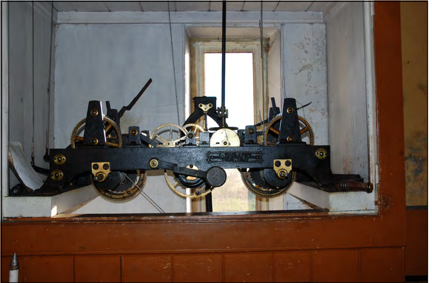
Plate 100: Second Floor: Room S04: clock mechanism and window W32. The pendulum attached to the mechanism extends into first floor room F04
