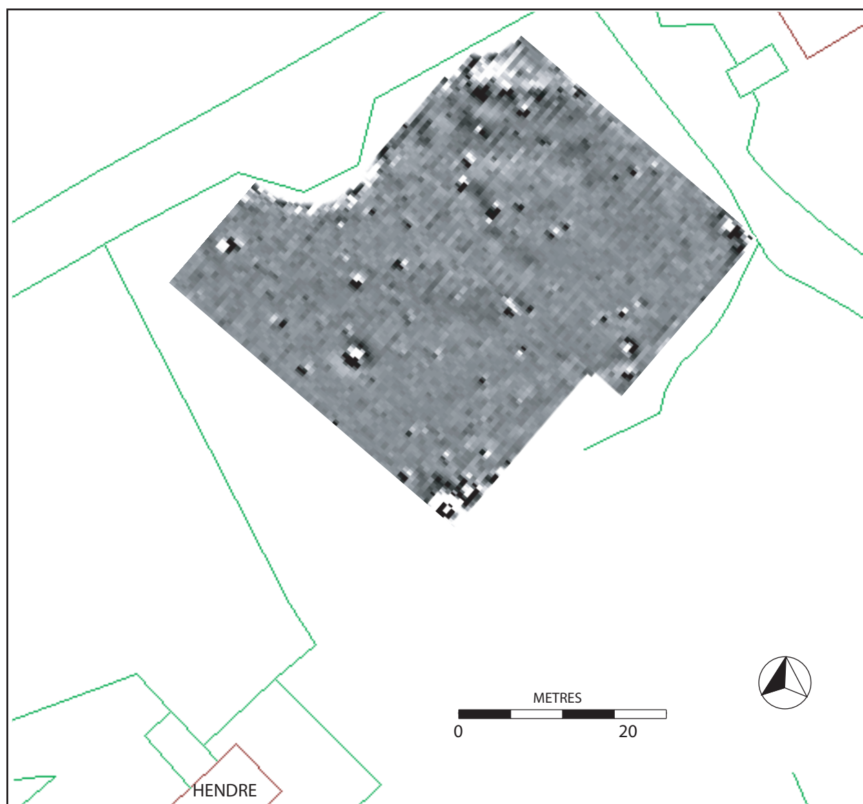
Fig. 3 Hendre Bach gradiometer survey - Processed data
