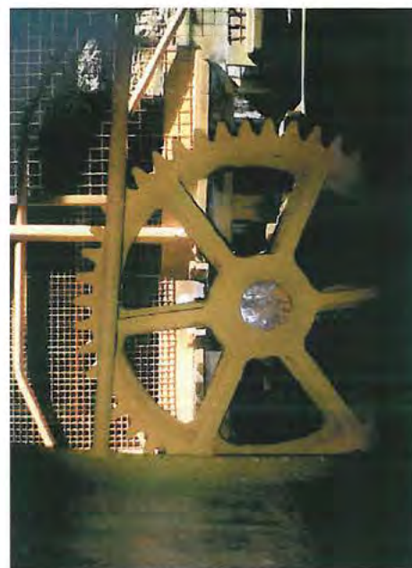
Plate 8 : The pinion wheel before remedial work. Note differential wear on teeth.
