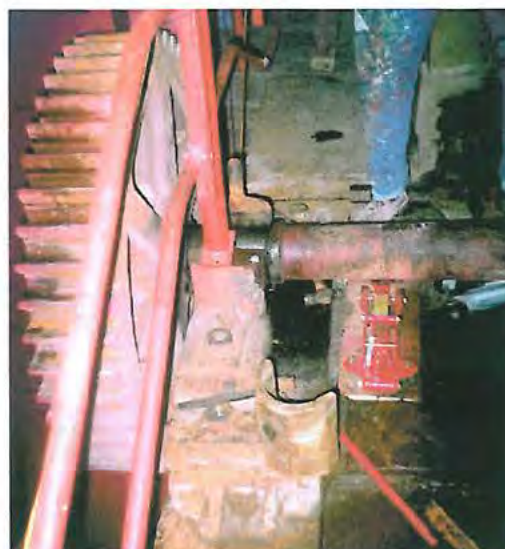
Plate 9 : Reversing the bearings supporting the pinion wheel and releveling the shaft.
