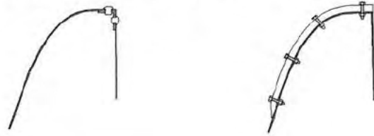
Fig 4 : Sectional view of the bucket construction and method of fixing
