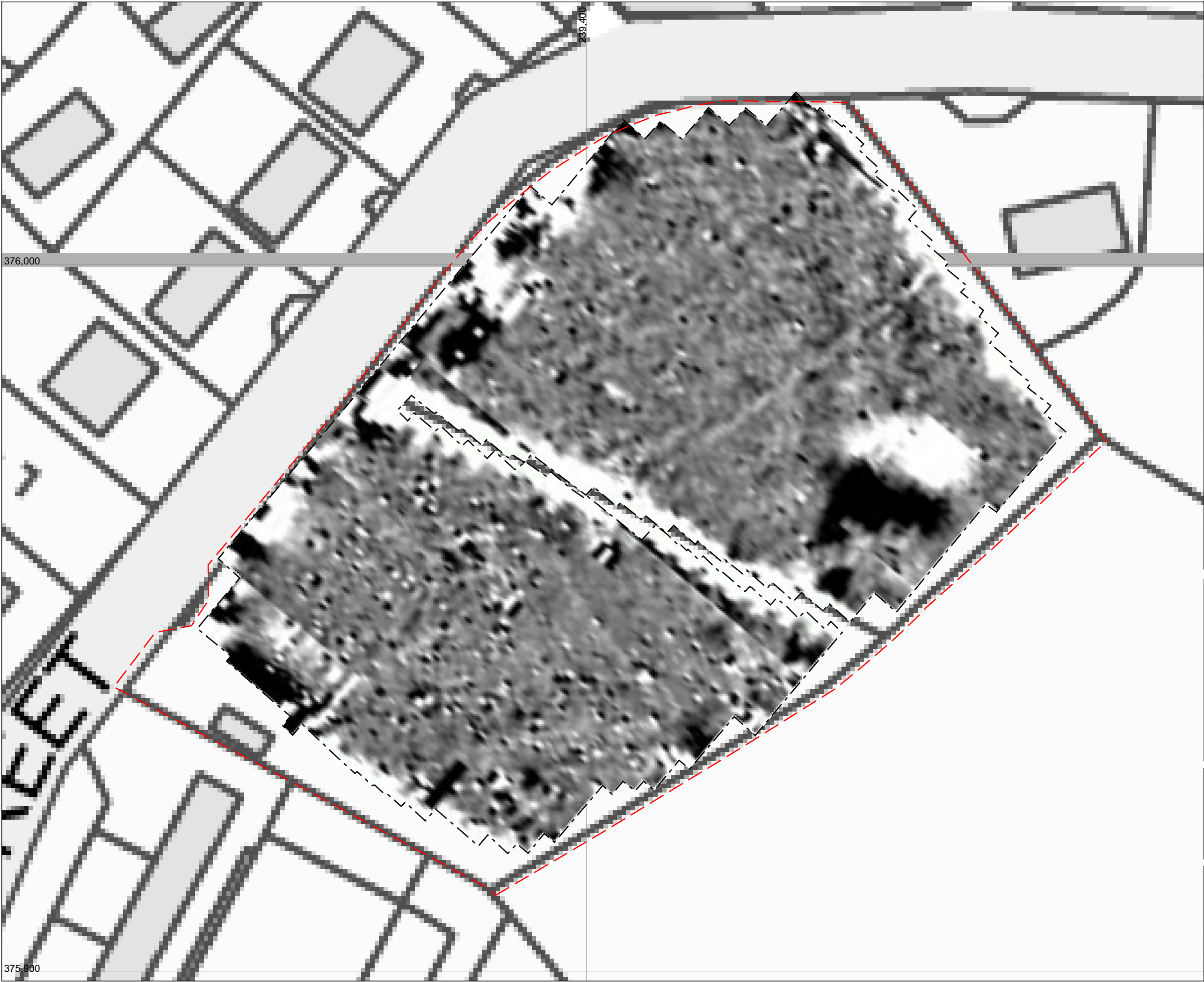
Figure 09: Geophysical survey processed greyscale plot (raw data clipped to +/- 15nT and de-stripped)
