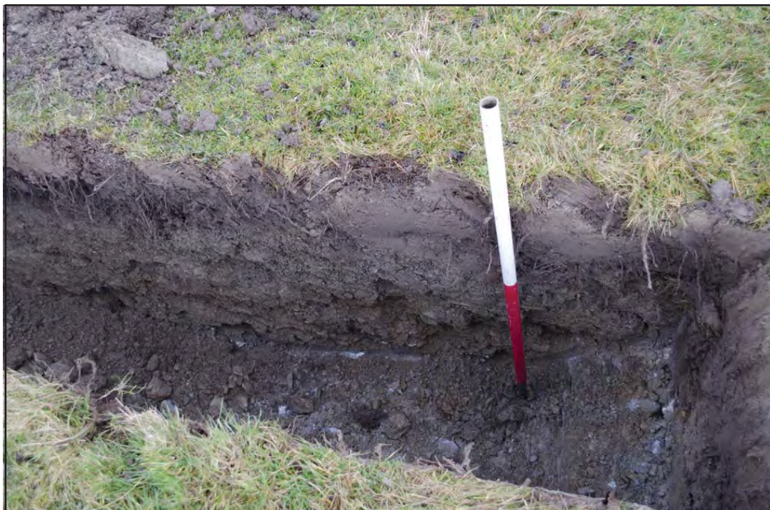
Plate 03: Trial Hole 1 - west facing section of Trial Hole 1 on encountering of glacial horizon at 1.3m; scale: 1.0m (archive image: G2492_017)
