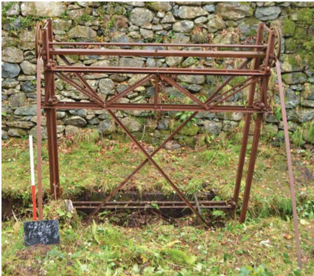
Plate 28. Left: Hythe pattern target frame at Penmaenucha rifle range (PRN 58671), right: elevation of Hythe pattern target frame (from Ministry of Defence, 2011, chapter 15, p21)
