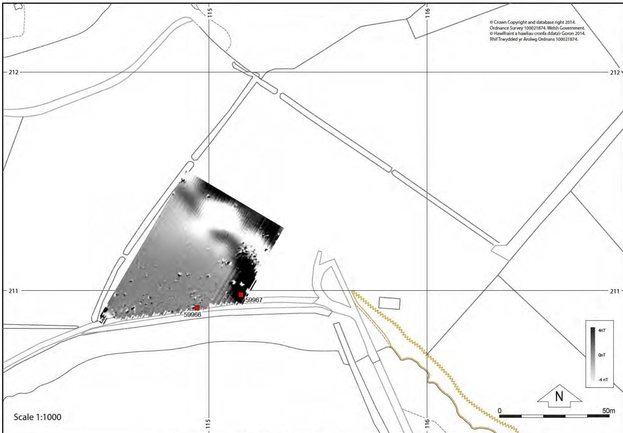
Figure 11. Area 3: West of Cefn Enlli, fluxgate gradiometer survey, grey-scale plot showing effects of buried geology
