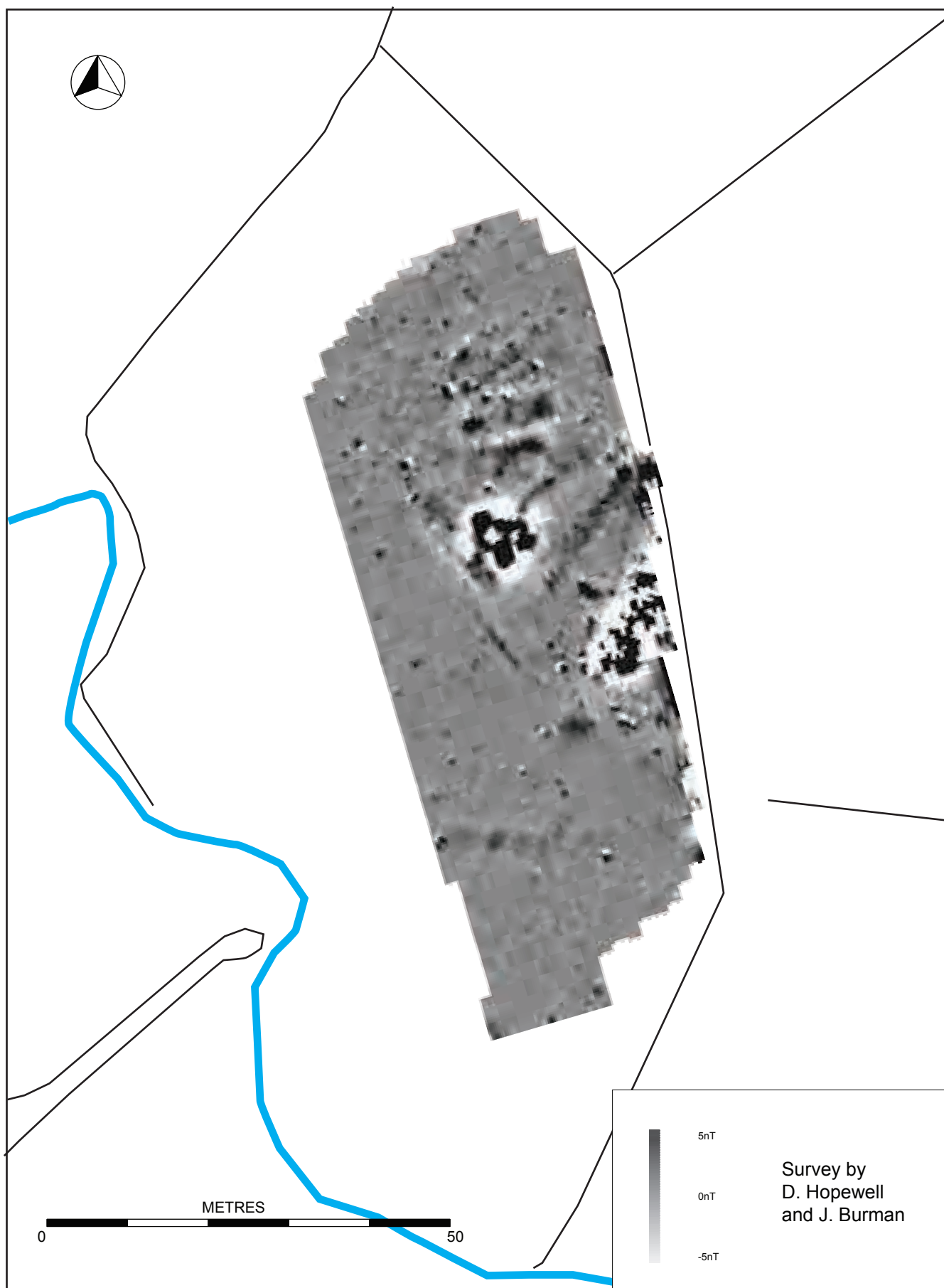
Fig. 10 Capel Euddog fluxgate gradiometer survey, grey scale plot
