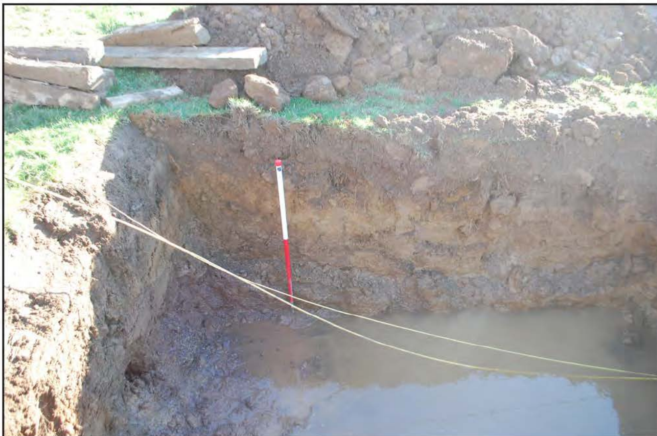
Plate 7: Pit 6/Field 5 - West facing section detailing topsoil, subsoil and disturbed ground associated with 1960's water main which is visible on the left of the picture. The base of the pit is waterlogged. Scale = 1 metre.
