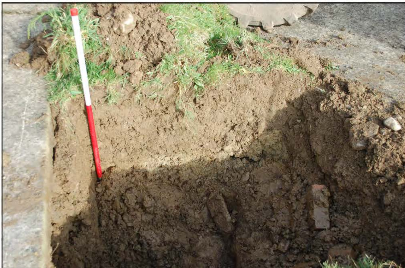
Plate 2: southern reservoir compound/pit 2 - south facing section detailing topsoil and disturbed subsoil with building debris. Scale = 1 metre.
