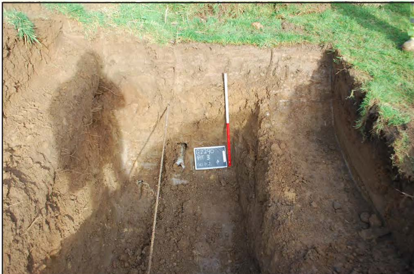
Plate 3: Pit 3/Field 2 - South facing section, detailing topsoil, subsoil, natural and existing 1960's main. Scale = 1 metre.
