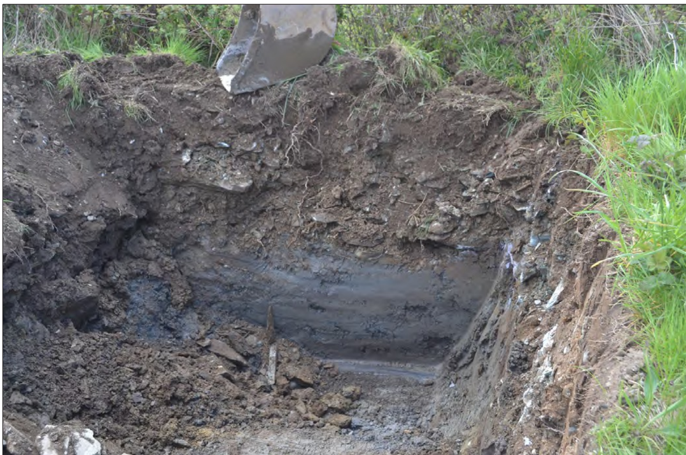
Plate 02: Trial hole 01 on the verge of the A487, shows material for the built up ground for the existing A487 road. The ground drops dramatically to the S. View from the N.
