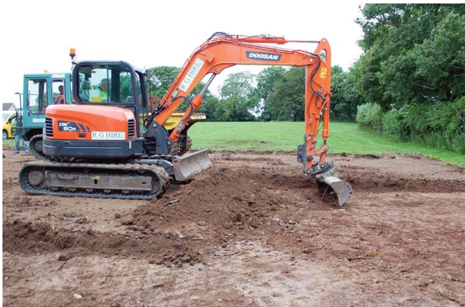
Plate 1. 18 tonne mechanical excavator stripping ploughsoil from the trench
