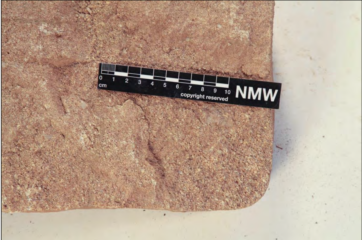
Figure 7: Specimen 24 8 - 5 of 9: Very well rounded corner of block showing evidence of working by hand
