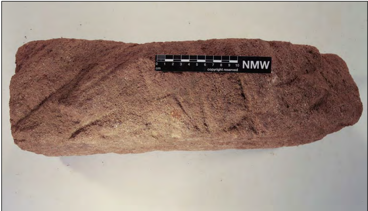
Figure 5: Specimen 40_9 - 5 of 5: Obvious 'tool marks' observed in face of block (nearest viewer) NB these may be masonry marks, or alternatively the result of plough damage
