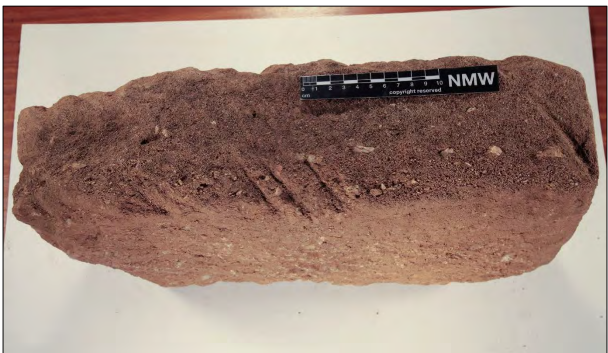
Figure 4: Specimen 40_9 - 3 of 5: Pebble rich horizon in lower half of block and tool marks on lateral surface (nearest viewer).
