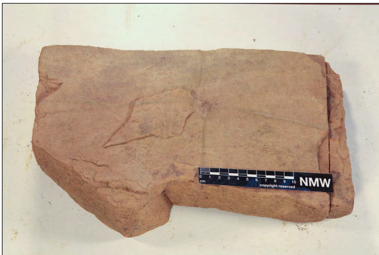
Figure 11: Specimen 71 25 3 of 3: Fragment splitting away from main block leaving very straight edge
