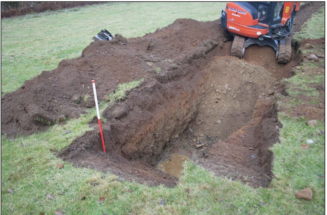
Plate 4: Angled view showing 101 - 103 and lower glacial layers to a depth of 3m; scale 1x1m; view from E (archive reference: G2665_010).
