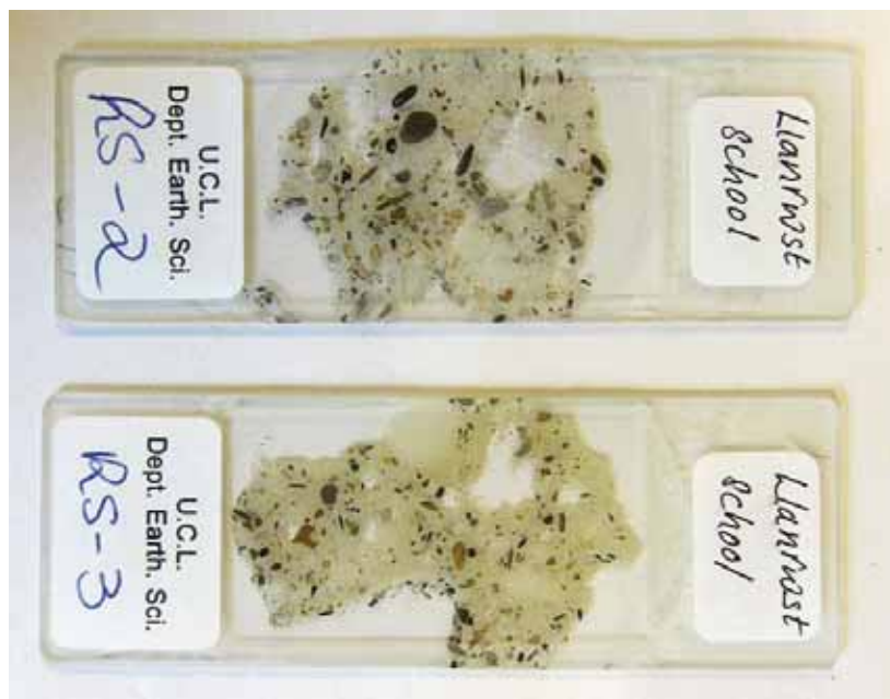
Samples of the School mortar mounted on microscope slides (76 x 26 mm) showing the macroscopic texture of these materials.
