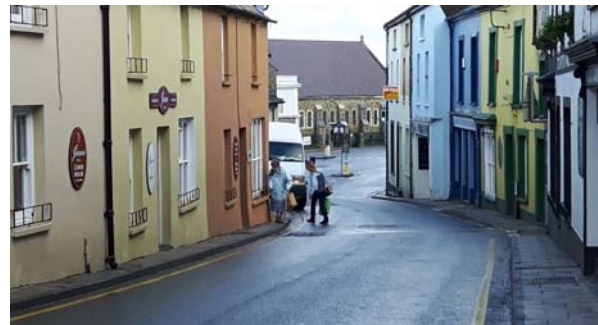
Figure 3-2 Narrow Footway Looking East along High Street forcing pedestrians into carriageway at the carriageways narrowest point and on a section with below standard visibility
