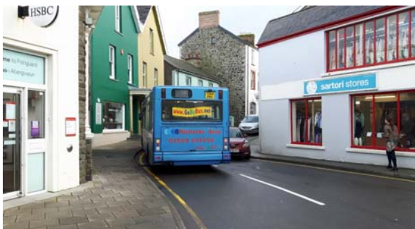
Figure 3-5 Narrow carriageway West Street approach to the Square causing vehicles to use both lanes and overhang of bus in footway
