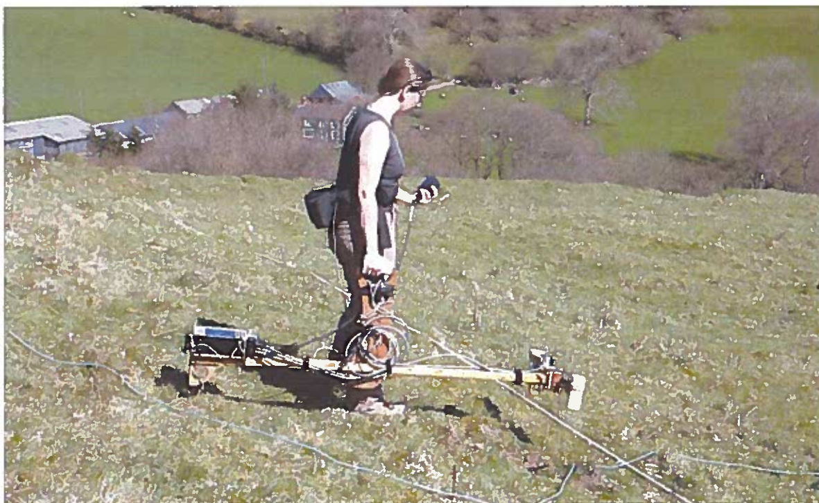
Figure 5. Anne Roseveare of Archaeophysica undertaking caesium magnetometry at Castell Grogwynion, March 2012 (Crown Copyright RCAHMMW).
