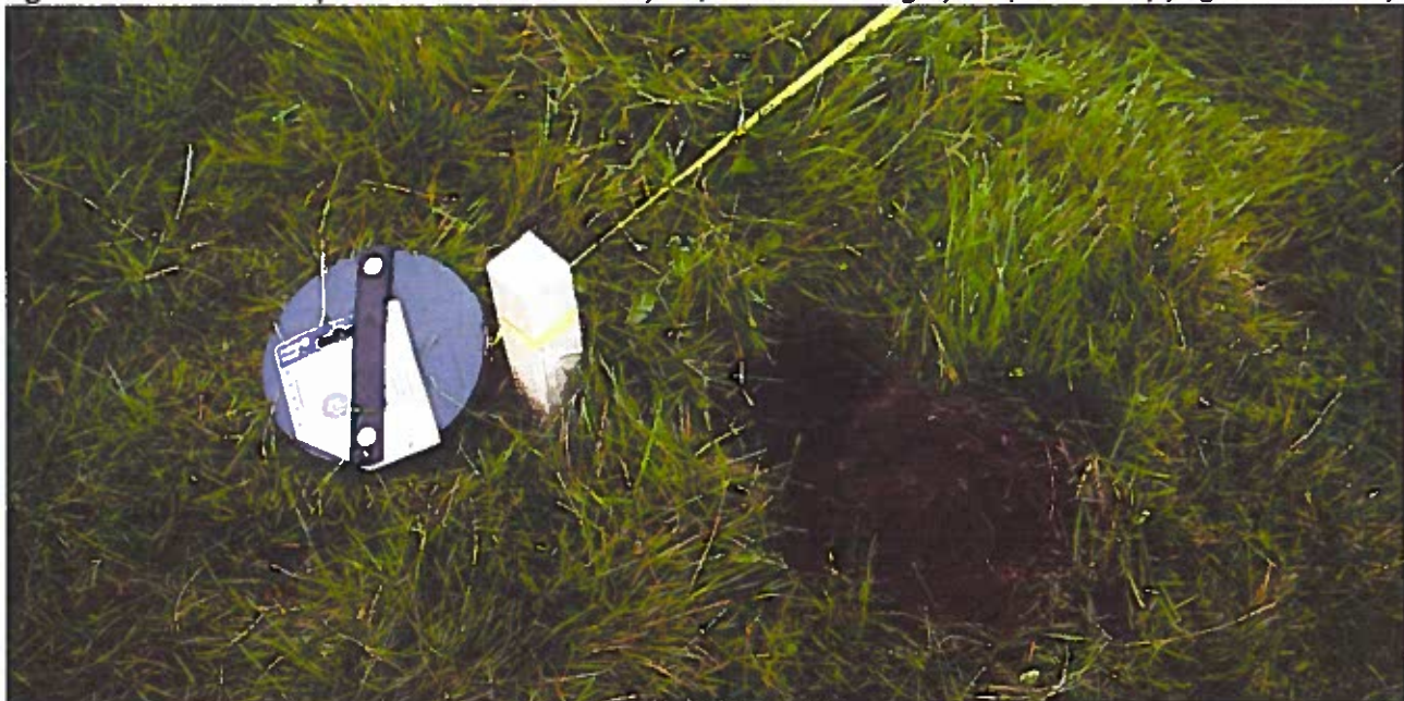
Figure 3. Sampling in progress at Darren Camp (north-west outer terrace) showing peg line marking sampling point, and standard 7-10cm turf removal to subsoil depth for sampling. Turf square is 'hinged' up for easy reinstatement (Crown Copyright RCAHMMW).
