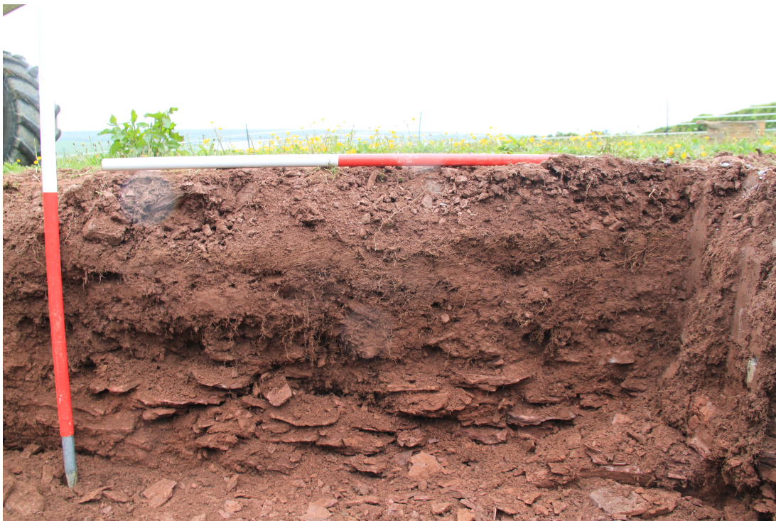
Plate 16 - AD003-D3-016 - Section of soil layers for septic tank trench at south end of site.
